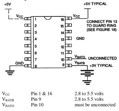
To always allow communication through the 1-Wire or wire port, the voltage on  $V_{CC}$  must be approximately 3-wire port, the voltage on  $V_{CC}$  must be approximately 0.2V above the voltage on  $V_{BATB}$ . Otherwise the DS2404 will retain data, but will not allow any access.
