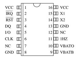
16-PIN DIP (300 MIL) 16-PIN SOIC (300 MIL) 16-PIN SSOP (300 MIL)
