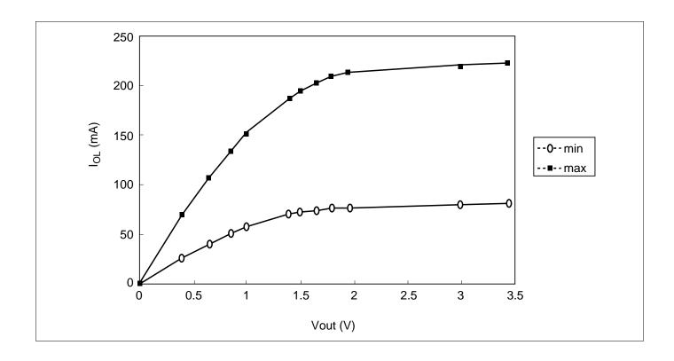
Output High Current ( $I_{OH}$ ) ( $Ta=0\ to\ +70^{\circ}C,\ V_{CC},\ V_{CC}Q=3.0\ V\ to\ 3.45\ V,\ V_{SS},\ V_{SS}Q=0\ V$ )
