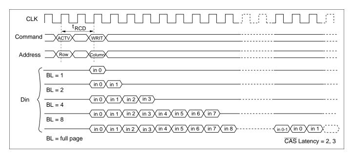
**2. Single write:** A single write operation is enabled by setting OPCODE (A9, A8) to (1, 0). In a single write operation, data is only written to the column address (AY0 to AY8; HM5212165F, AY0 to AY9; HM5212805F) and the bank select address (A12/A13) specified by the write command set cycle without regard to the burst length setting. (The latency of data input is 0 clock).
