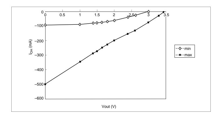
**DC Characteristics** (Ta = 0 to +70°C,  $V_{CC}$ ,  $V_{CC}Q = 3.3 \text{ V} \pm 0.3 \text{ V}$ ,  $V_{SS}$ ,  $V_{SS}Q = 0 \text{ V}$ ) (HM5212165F)
