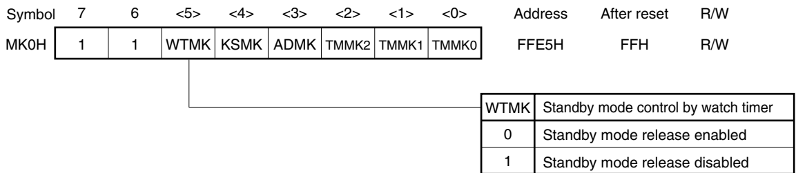
Figure 16-19. Format of Interrupt Mask Flag Register 0H
