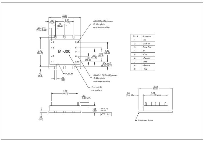
Note: For alternate package options refer to the mechanical drawing page of vicorpower.com
