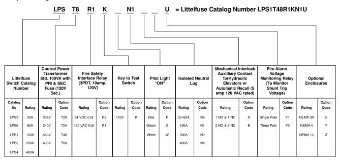
**Note:** Desired options must appear in the order shown above. Typical options include Control Power Transformer, Fire Safety Interface Relay, Mechanical Interlock Auxiliary Contact and Fire Alarm Voltage Monitoring Relay.
