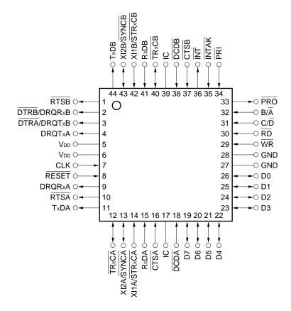
IC: Internally Connected (Leave this pin unconnected)
