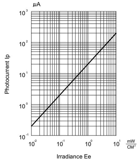
Fig.6 PHOTOCURRENT VS IRRADIANCE  $\lambda = 940 \text{ nm}$
