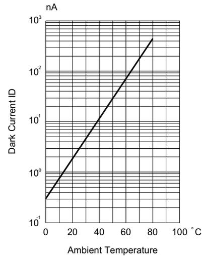
Fig.4 DARK CURRENT AMBIENT TEMPERATURE
