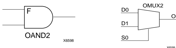
Figure 20: AND & MUX Symbols in XC4000X IOB
