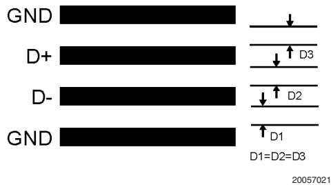
FIGURE 10. Ideal Diode Trace Layout
