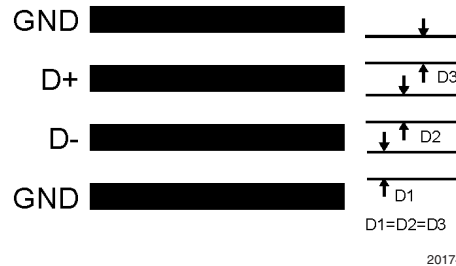
FIGURE 8. Ideal Diode Trace Layout
