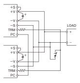
Figure 3-4: Parallel Operation which is possible to adjust output voltage by external applied voltage
