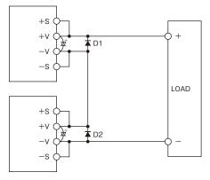
Figure 12-1: Series Operation for High Output Voltage Configurations
