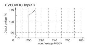
Figure 2-1: Limitation of Input Voltage Range
