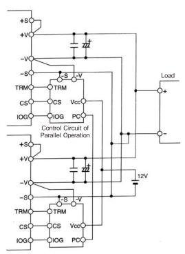
Control Circuit of Parallel Operation
