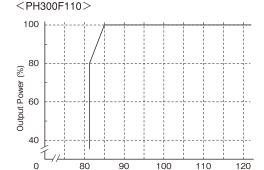
Figure 1-1: PH110 Series Output Derating
