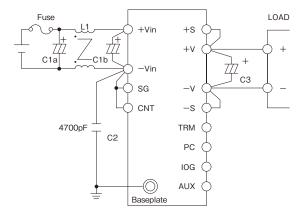
Figure 1-3: Basic Connection Circuit
