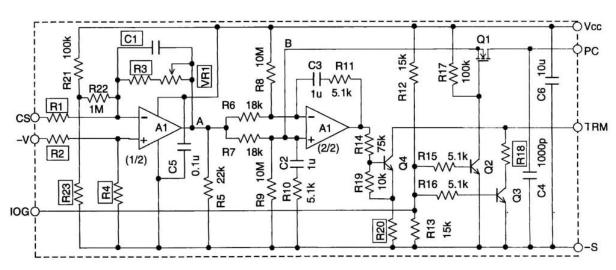
Figure 3-2 Control Circuit fo Parallel Operation
