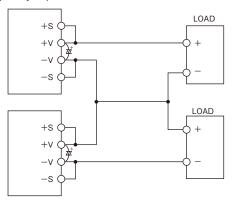
Figure 12-2: Series Operation using ± Output
