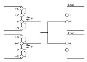
Figure12-2 ±Output Series Operation
