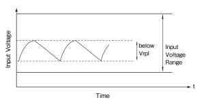
Figure 1-1 Ripple Voltage
