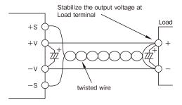
Figure9-1 Remote Sensing at Use
