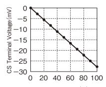
Output Current(%) Figure 3-3 Characteristics of Output Current vs. CS Terminal Voltage (Example: PH300S48-5)
