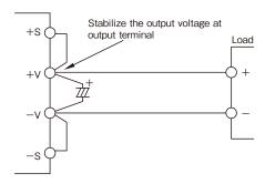
Figure9-2 Remote Sensing Not in Use
