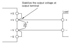
Figure 9-2: Without Remote Sensing
