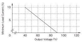
Figure2-6: Minimum Output Current Limit
