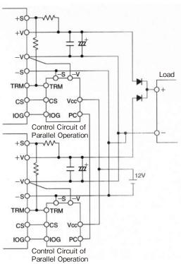
Figure6-2 N+1 Redundant Operation at programmed output voltage (fixed)
