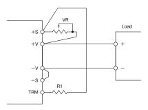
Figure 2-2 Example Connection of External Resistance
