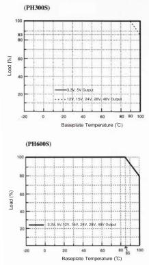
Figure14-1Output Derating Curve
