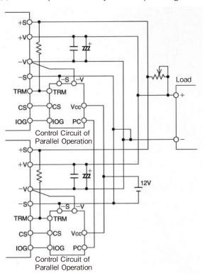
Figure5-3 Parallel Operation with adjustable output voltage
