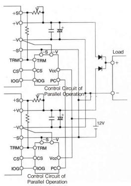
Figure 6-3 N+1 Redundant Operation with adjustable output voltage
