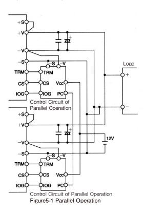
(b) Parallel Operation programmed output voltage
