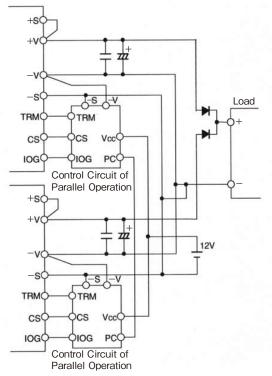
Figure 6-1 N+1 Redundant Operation
