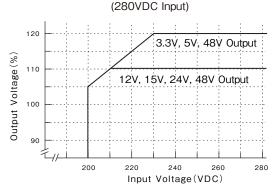
Figure 2-1 Limit of Input Voltage
