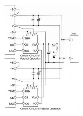
Figure 3-5 Example: Vcc is supplied by +V
