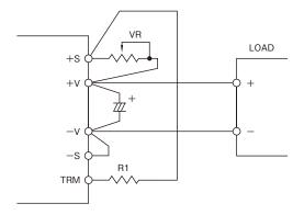
Figure2-4: Connection Example of External Resistor Network #3 PH100S/PH150S
