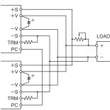
Figure 3-3: Parallel Operation with adjustable voltage
