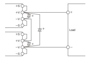
Figure 12-1 Series Operation in High Output Voltage
