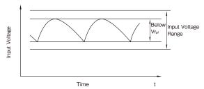
Figure 1-2: Input Ripple Voltage
