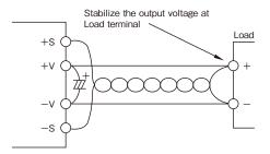
Figure9-1: Using Remote Sensing
