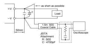
Figure 3-1 Measurement of Maximum Output Ripple & Noise (Example: PH300S)
