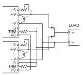
Figure4-3: N+1 Redundant Operation with adjustable output voltage
