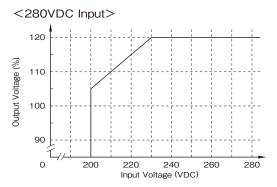
Figure2-5: Limitation of Input Voltage
