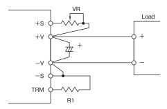
Figure 2-7: Connection Example of External Resistor
