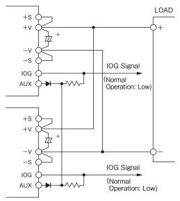
Figure 13-1: Example of IOG Terminal Connection
