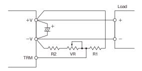
Figure2-2: Connection Example of External Resistor Network #1 (no ±S Terminal, PH50S/PH75S)
