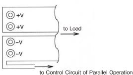
Figure 3-4 - V Wiring Example
