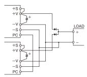
Figure 4-1: N+1 Redundant Operation
