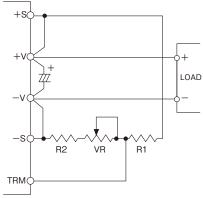
Figure2-3: Connection Example of External Resistor Network #2 (with ±S Terminal)
