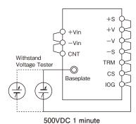
Figure 20-3 Withstand Voltage Test for Output - Baseplate
