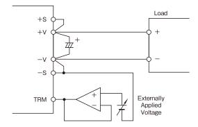
Figure 2-9: Example of Applied Voltage
