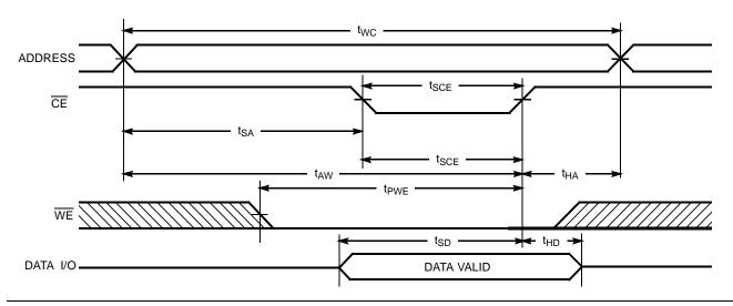
Write Cycle No. 2 (WE Controlled, OE HIGH During Write)[12, 13]
