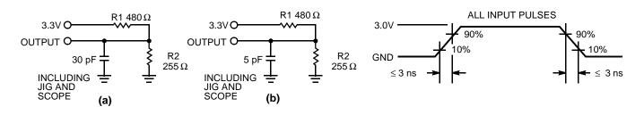
THÉVENIN EQUIVALENT Equivalent to: 167Ω **--O** 1.73V OUTPUT O
