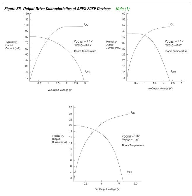
Figure 35 shows the output drive characteristics of APEX 20KE devices.
