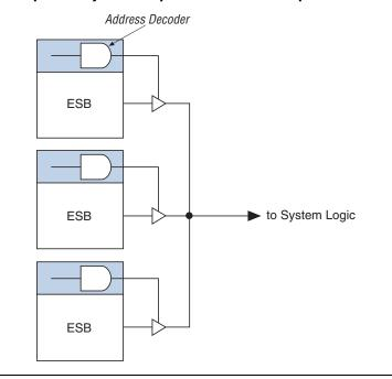
Figure 18. Deep Memory Block Implemented with Multiple ESBs
