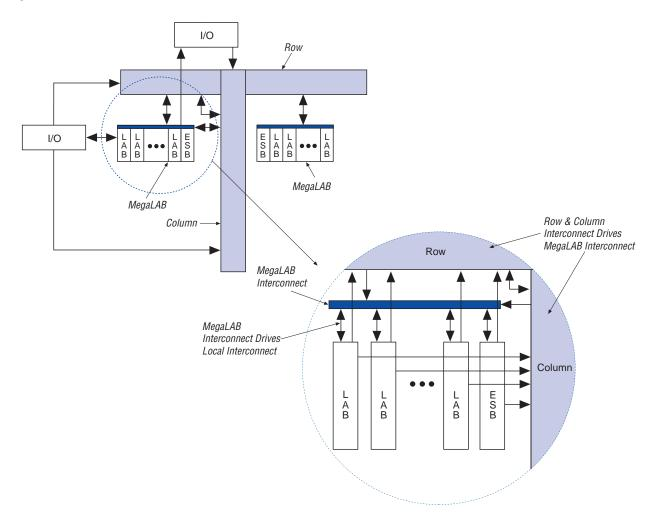
Figure 10. FastTrack Connection to Local Interconnect
