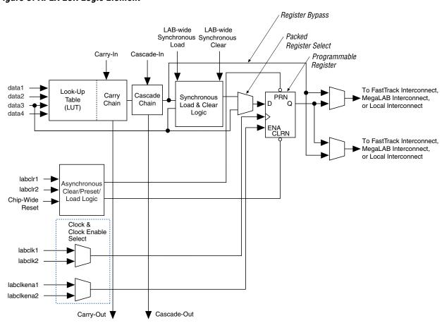
Figure 5. APEX 20K Logic Element
