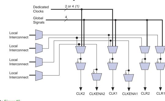
Figure 15. ESB Product-Term Mode Control Logic
