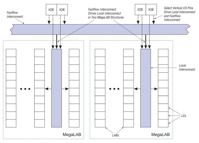
Figure 12. APEX 20KE FastRow Interconnect
