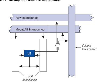
Figure 11. Driving the FastTrack Interconnect
