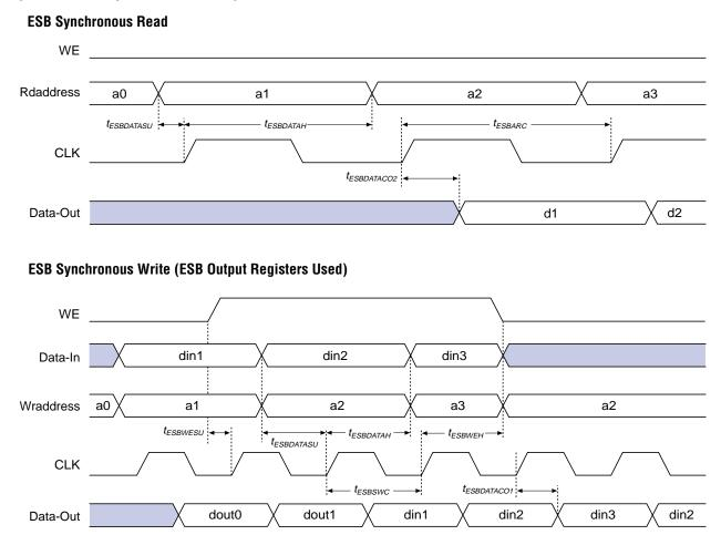
Figure 39. ESB Synchronous Timing Waveforms
