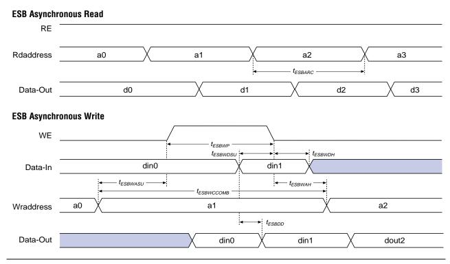
Figure 38. ESB Asynchronous Timing Waveforms
