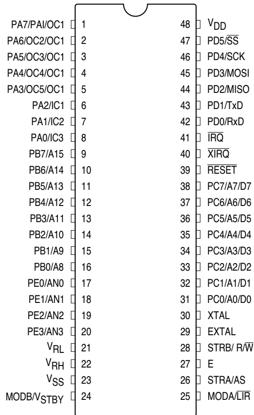
Figure 3 48-Pin DIP Pin Assignments
