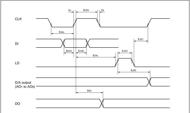
Note : The D/A output evaluation level is 90% and 10% of Vcc. The other evaluation level is 80% and 20% of Vcc.
