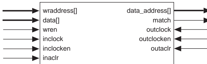
Figure 23. APEX 20KE CAM Block Diagram
