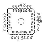
**Figure 1. Programming Pinouts**
