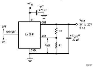
$$\begin{split} V_{OUT} &= \text{Reference voltage} \times \frac{\text{R1} + \text{R2}}{\text{R1}} \text{ where } V_{\text{REF}} = 1.275 \text{ typical} \\ \text{Solving for R2: } \text{R2} &= \text{R1} \left( \frac{V_{O}}{V_{\text{REF}}} - 1 \right) \end{split}$$
