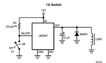
\*\*\* To assure shutdown, select Resistor R3 to guarantee at least 300µA of pull-up current when S1 is open. (Assume 2V at the ON/OFF pin.)
