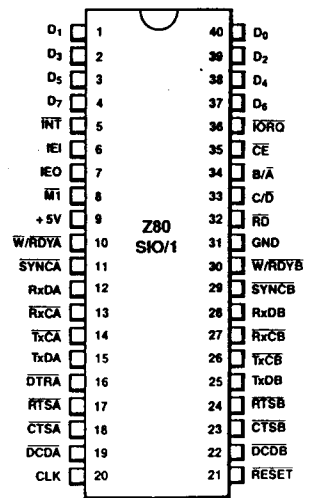
Figure 4. 40-pin Dual-In-Line Package (DIP), Pin Assignments
