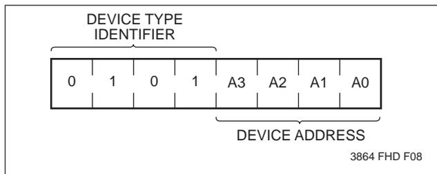
The next four bits of the slave address are the device address. The physical device address is defined by the state of the A0-A3 inputs. The X9241 compares the serial data stream with the address input state; a successful compare of all four address bits is required for the X9241 to respond with an acknowledge.
