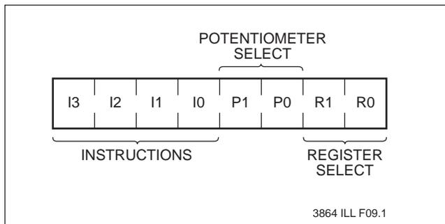
The four high order bits define the instruction. The next two bits (P1 and P0) select which one of the four potentiometers is to be affected by the instruction. The last two bits (R1 and R0) select one of the four registers that is to be acted upon when a register oriented instruction is issued.
