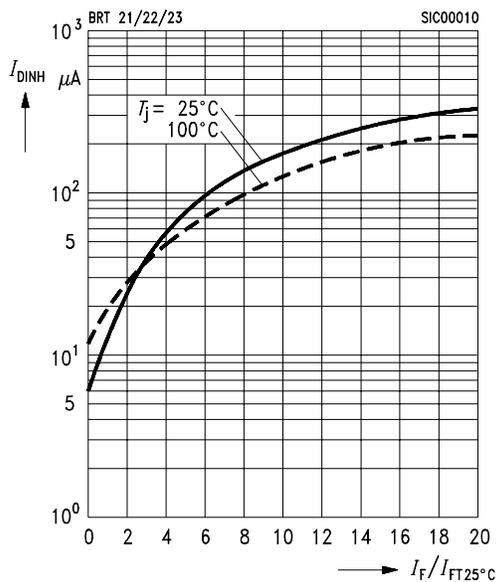
**Typ. static inhibit voltage limit**  $V_{DINHmin} = f(I_F/I_{FT 25^\circ C})$ , parameter:  $T_j$
