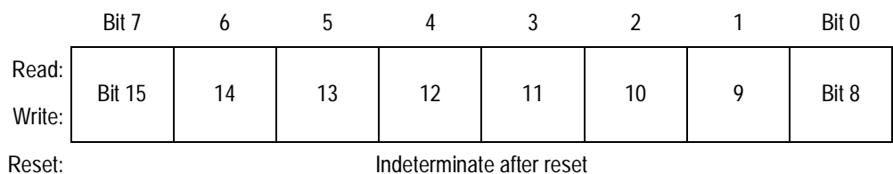
Figure 22-9. TIMA Channel Registers (TACH0H/L–TACH3H/L) (Sheet 1 of 3)
