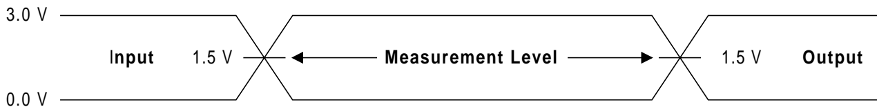
Figure 14. Input Waveforms and Measurement Levels
