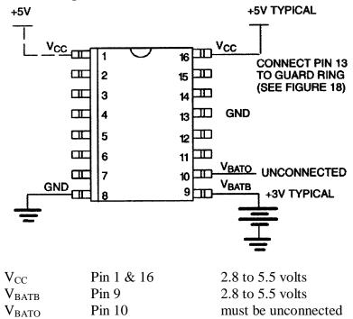
To always allow communication through the 1-Wire or wire port, the voltage on  $V_{CC}$  must be approximately 3-wire port, the voltage on  $V_{CC}$  must be approximately 0.2V above the voltage on  $V_{BATB}$ . Otherwise the DS2404 will retain data, but will not allow any access.
