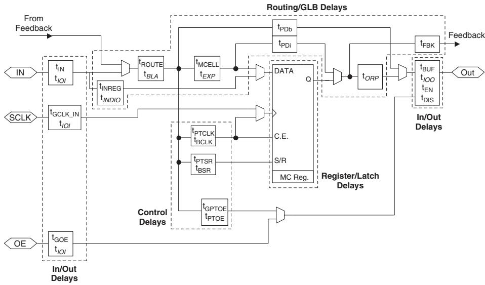
**ispMACH 4000V/B/C Internal Timing Parameters**
