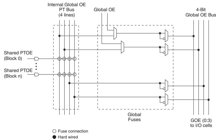
**Figure 10. Global OE Generation for ispMACH 4032**
