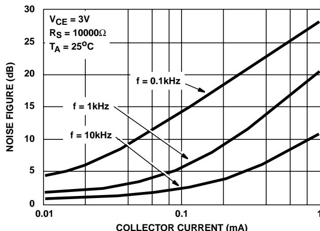
**FIGURE 10. TYPICAL NOISE FIGURE vs COLLECTOR CURRENT**
