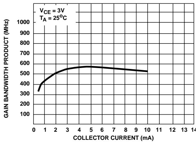
**FIGURE 16. TYPICAL GAIN BANDWIDTH PRODUCT vs COLLECTOR CURRENT**
