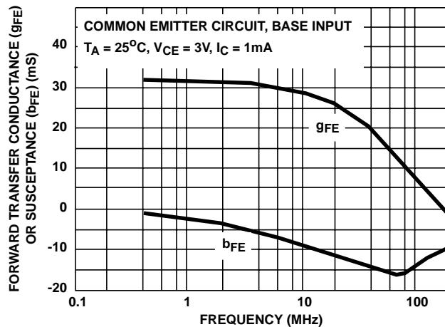
**FIGURE 12. TYPICAL FORWARD TRANSFER ADMITTANCE vs FREQUENCY**
