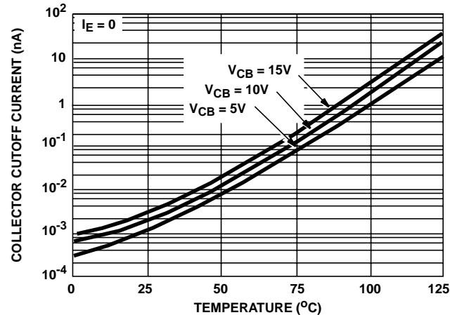
FIGURE 1. TYPICAL COLLECTOR-TO-BASE CUTOFF CURRENT
