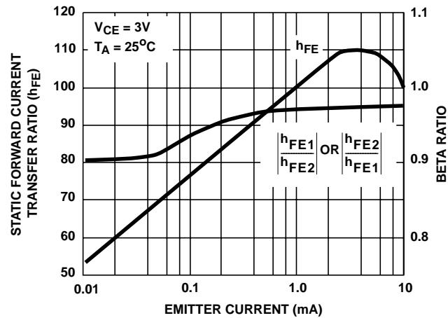
FIGURE 3. TYPICAL STATIC FORWARD CURRENT TRANSFER
