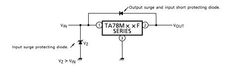
(3) When the input voltage is too high, the power dissipation of three terminal regulator increases because of series regulator, so that the junction temperature rises. In such a case, it is recommended to reduce the power dissipation by inserting the power limiting resistor R<sub>SD</sub> in the input terminal, and to reduce the junction temperature as a result.
