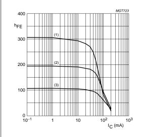
**BC846A**;  $V_{CE} = 5 \text{ V}$ .
