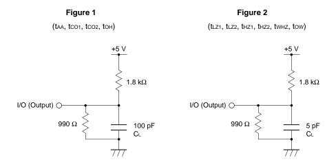
Remark CL includes capacitance of the probe and jig, and stray capacitance.
