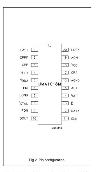
225 mV (RMS), and at frequencies as high as 1.25 GHz. The high frequency divider circuits use bipolar transistors, slower bits are CMOS. Divider ratios (512 to 131 071) allow a 1 MHz phase comparison with a 500 MHz RF input, and a 10 kHz phase comparison with a 1.25 GHz RF input.
