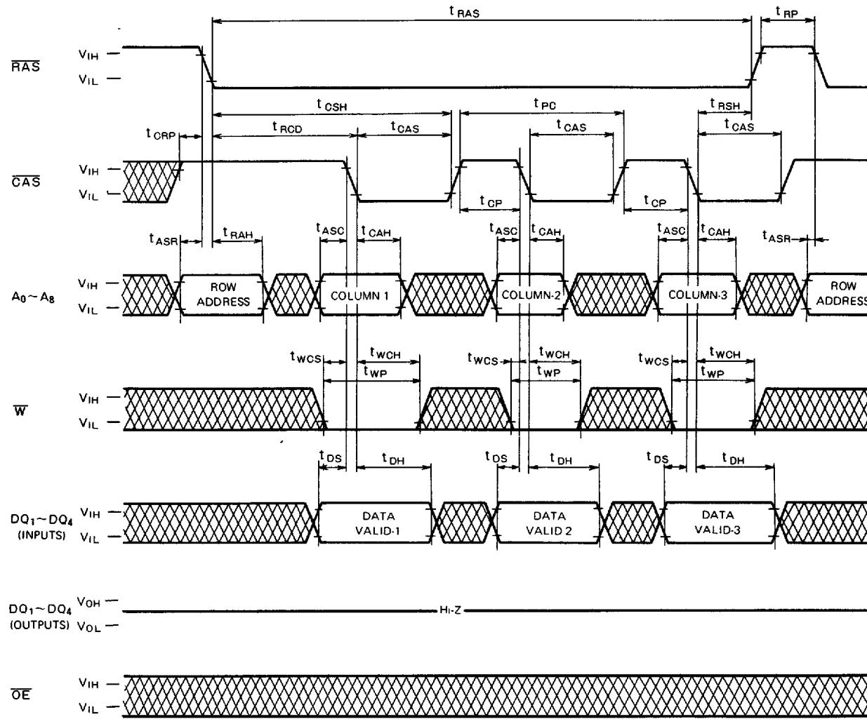
**FAST PAGE MODE 1048576-BIT(262144-WORD BY 4-BIT) DYNAMIC RAM****Fast Page Mode Write Cycle (Delayed Write)**
