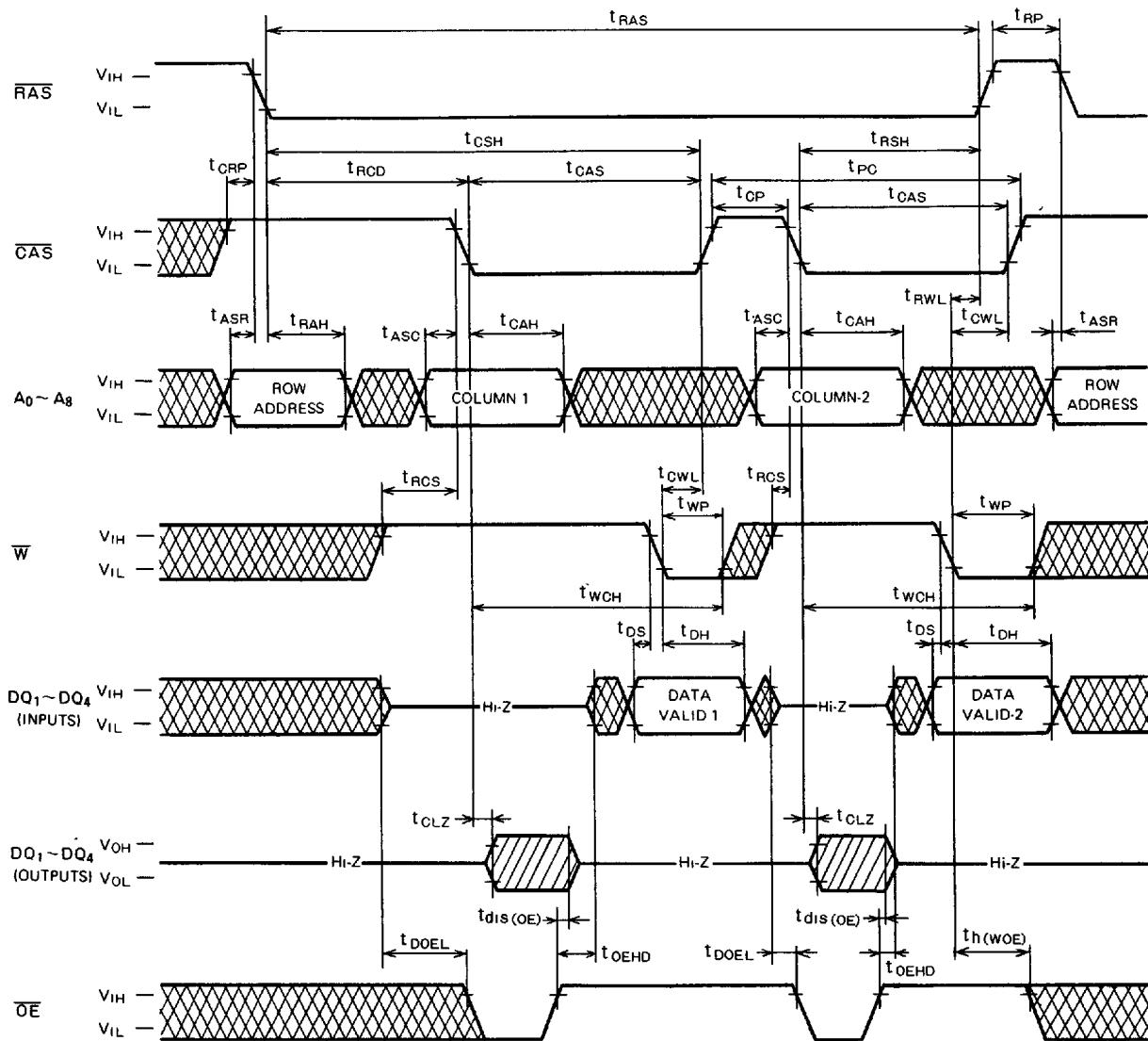
**FAST PAGE MODE 1048576-BIT(262144-WORD BY 4-BIT)DYNAMIC RAM****Fast Page Mode Read-Write, Read-Modify-Write Cycle**
