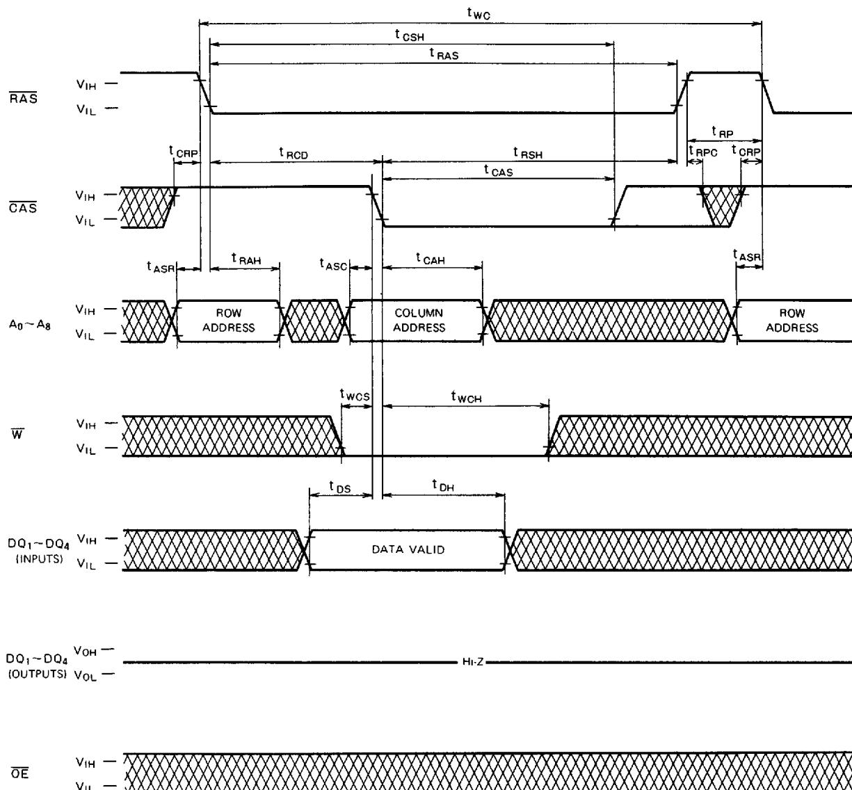
**FAST PAGE MODE 1048576-BIT(262144-WORD BY 4-BIT)DYNAMIC RAM****Write Cycle (Delayed Write)**
