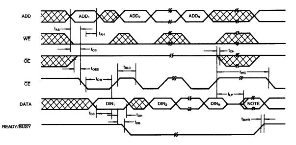
\* NOTE:  $I/O_7$  output  $\overline{DIN_N}$  when the chip is read.  $I/O_6$  is toggling between "1" and "0" when the chip is successively read.
