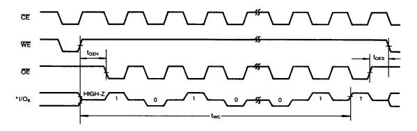
\* During the write cycle, I/O<sub>6</sub> will toggle between "1" and "0".
