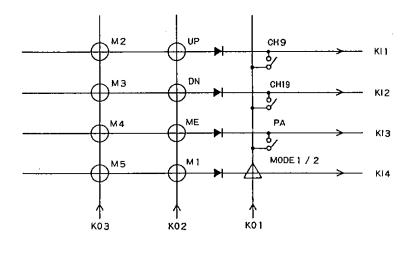
CH9 : Emergency CH 9 recall CH19 : Emergency CH19 recall PΑ : Public announcement display MODE 1 / 2 : Display Mode UP : CH up/scan DΝ : CH down/scan : Station Memory Enable ME  $M1 \sim M5$ :Station Memory recall
