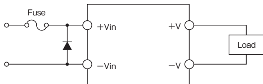
Figure1-5: Protection for Reversed Connection of Input
