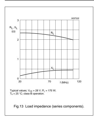
**OPERATING NOTE** for Figs 12, 13 and 14: Below 50 MHz a base-emitter resistor of 4,7  $\Omega$  is recommended to avoid oscillation. This resistor must be effective for r.f. only.
