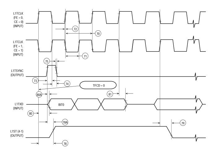
Figure 10-62. SI Transmit Timing with Normal Clocking (DSC = 0)
