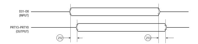
Figure 10-37. External MC68030/MC68360 Parity Bits Timing Diagram
