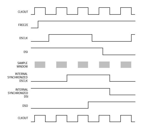
Figure 5-23. Serial InterfaceTiming Diagram
