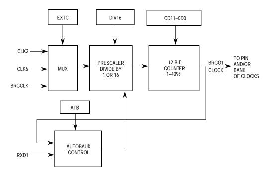
Figure 7-36. Baud Rate Generator Block Diagram
