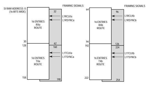
Figure 7-26. Two TDMs with Dynamic Frames
