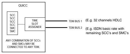
NOTE: Two TDM buses may be simultaneously supported with the time slot assigner.
