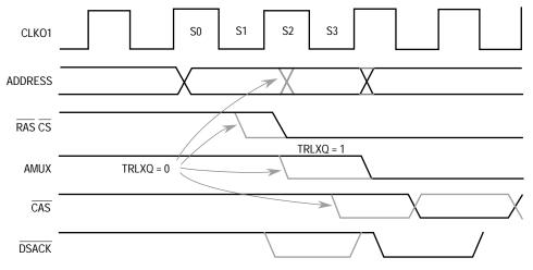
Figure 6-16. TRLXQ = 1 During an Internal Cycle
