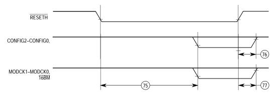
Figure 10-16. Configuration And Clock Mode Select Timing
