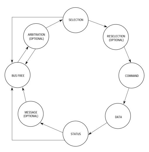
Figure 9-20. Phase Sequences of the SCSI Bus
