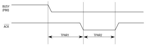
Figure 7-89. Centronics Receiver Timing Mode 0
