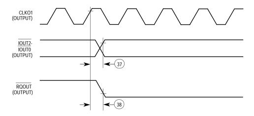
Figure 10-57. Slave Mode: Interrupts Timing Diagram
