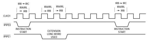
Figure 5-29. Instruction Pipeline Timing Diagram
