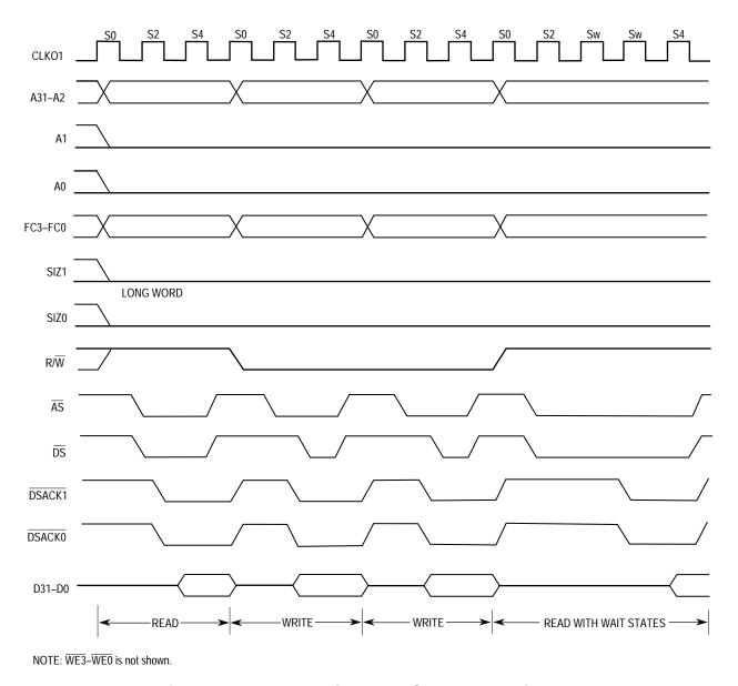
Figure 4-20. Read-Write-Read Cycles—32-Bit Port
