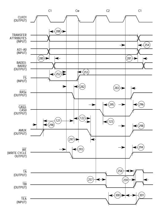
Figure 10-46. External MC68040 DRAM Cycles Timing Diagram
