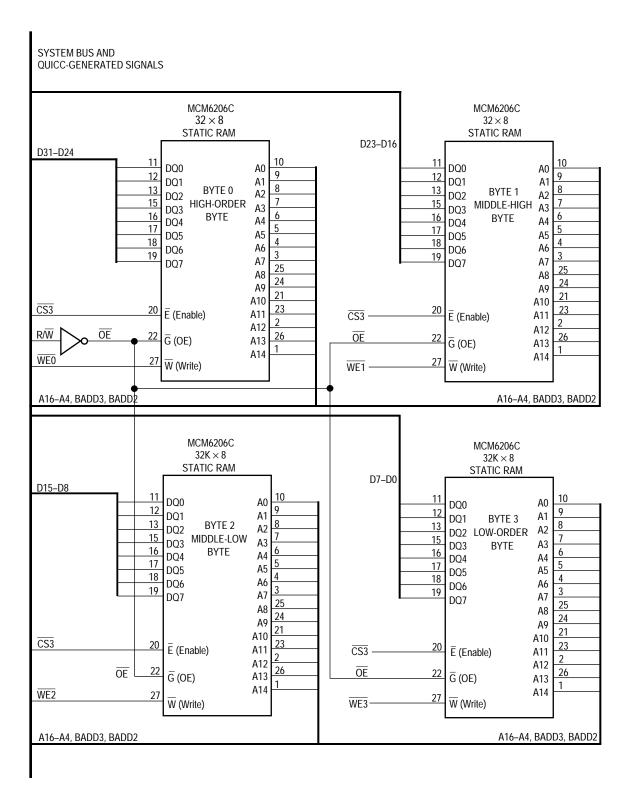
Figure 9-12. 128-Kbyte Static RAM Bank—32 Bits Wide
