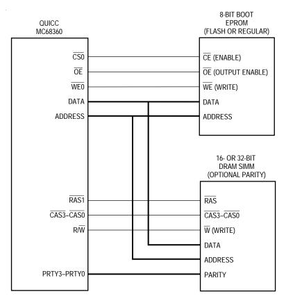
Figure 6-11. Minimum QUICC System Configuration
