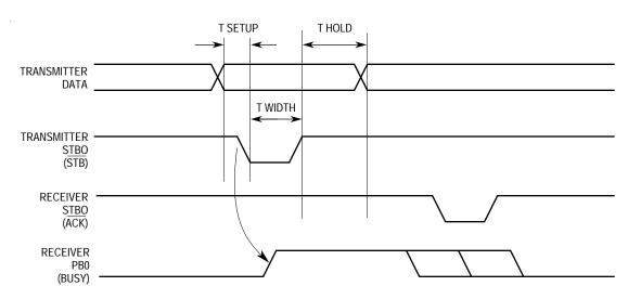
Figure 7-87. Pulsed Handshake Busy Signal
