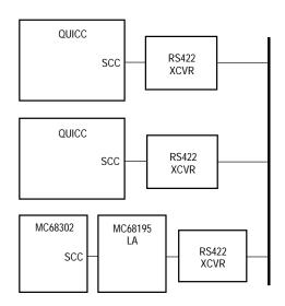
NOTE: The QUICC implements the AppleTalk LAN protocol without the need for the MC68195.
