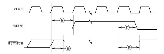
Figure 10-18. Background Debug Mode FREEZE Timing
