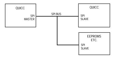
NOTE: Two QUICCs configured for a master-slave SPI connection.
