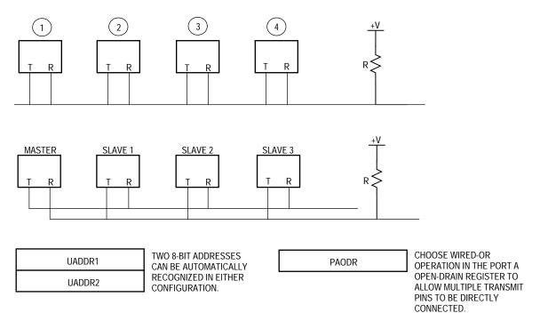
Figure 7-47. Two Configurations of UART Multidrop Operation
