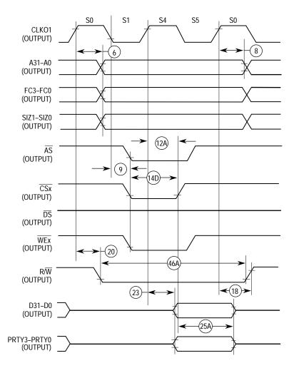
Figure 10-10. SRAM: Fast Termination Write Cycle (CSNTQ = 1)
