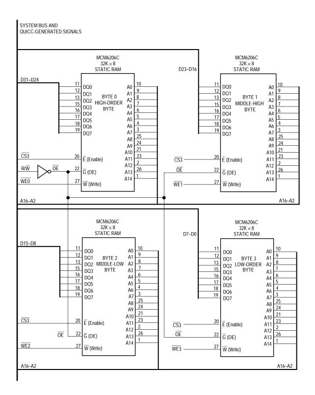
Figure 9-30. 128-Kbyte Static RAM Bank—32 Bits Wide
