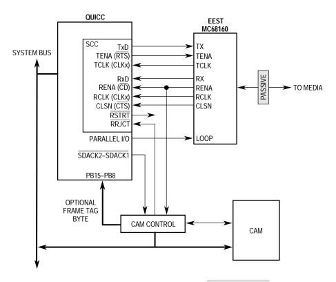
NOTE: The receive data is sent to the CAM as it is written to system memory. The SDACK2-SDACK1 signals are used to identify the destination address and any other frame bytes desired. The RSTRT signal is not required in this configuration, although it is still available.
