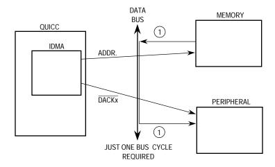
Figure 7-14. Single Address Transfer Example
