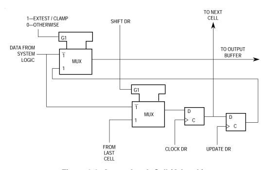
Figure 8-3. Output Latch Cell (O.Latch)
