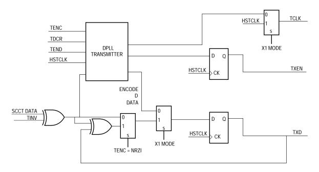
Figure 7-45. DPLL Transmit Block Diagram
