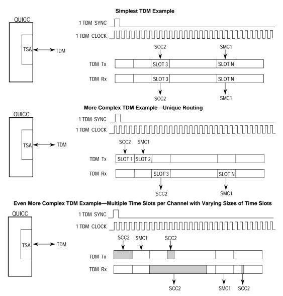
NOTE: The two shaded areas of SCC2 Rx are received as one high-speed data stream by SCC2 and stored together in the same data buffers.
