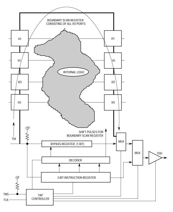
Figure 9-23. TAP Controller and Registers
