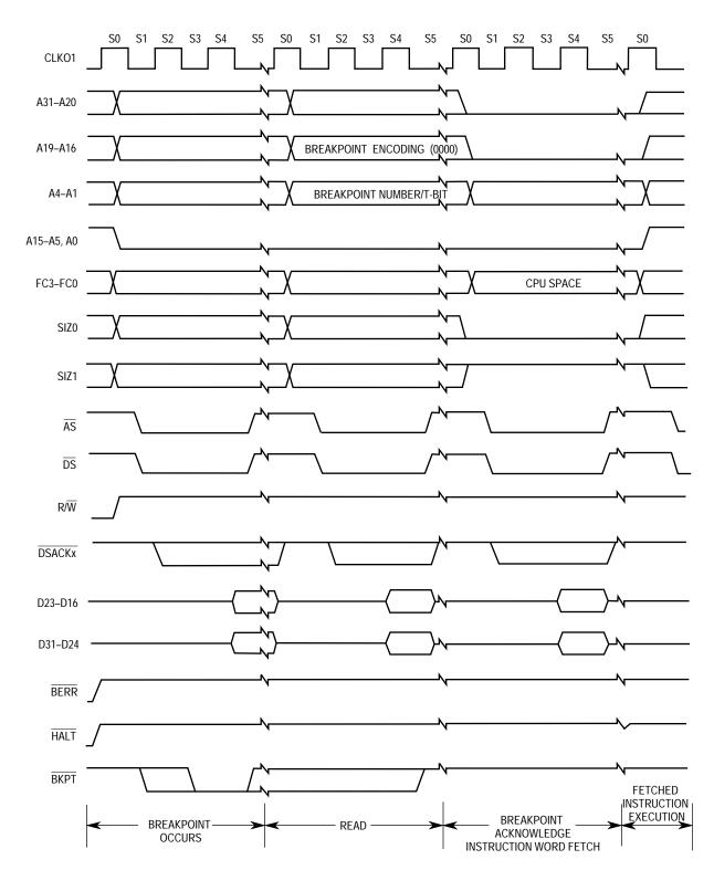
Figure 4-24. Breakpoint Acknowledge Cycle Timing (Opcode Returned)
