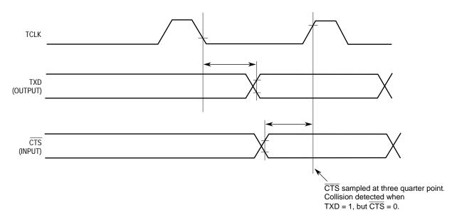
Figure 7-57. Non-Symmetrical Duty Cycle
