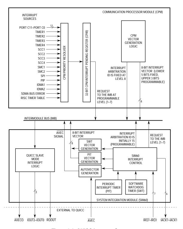
Figure 6-3. QUICC Interrupt Structure
