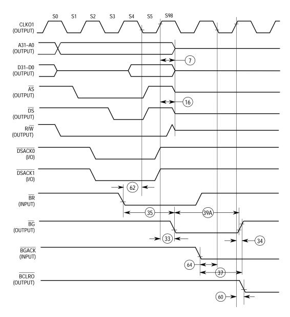
Figure 10-15. SYNC Bus Arbitration – Active Bus Case
