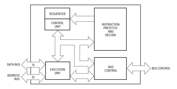
Figure 5-1. CPU32+ Block Diagram
