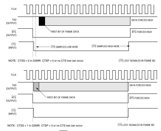
Figure 7-41. CTS Lost in Synchronous Protocols
