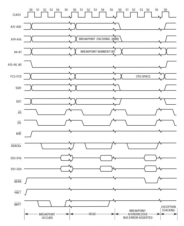
Figure 4-25. Breakpoint Acknowledge Cycle Timing (Exception Signaled)
