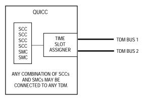
NOTE: Two TDM buses may be simultaneously supported with the time slot assigner.
