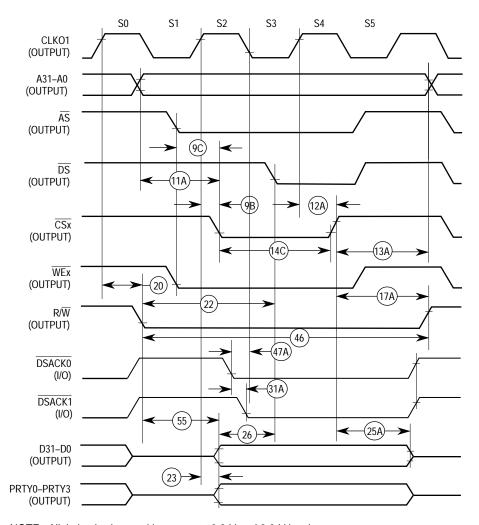
Figure 10-11. SRAM: Write Cycle (TRLX = 1, CSNTQ = 1, TCYC = 0)
