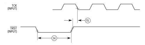
Figure 10-80. TRST Timing Diagram
