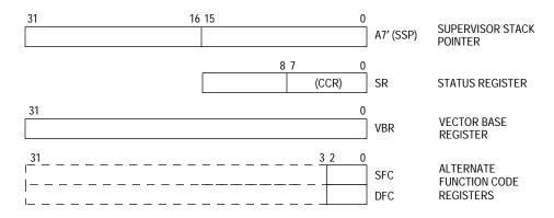
Figure 5-4. Supervisor Programming Model Supplement
