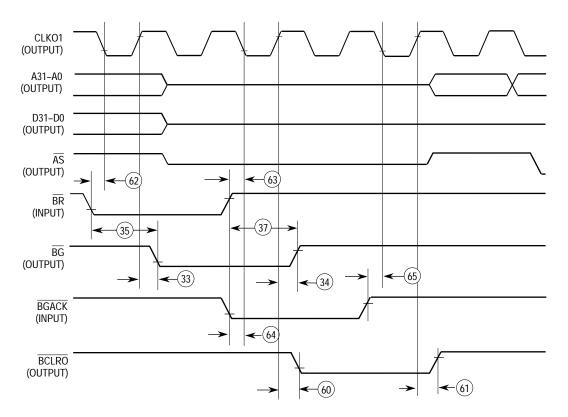
Figure 10-14. SYNC Bus Arbitration – IDLE Bus Case
