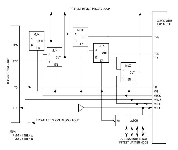
Figure 9-24. Signal Routing with TAP Port Used in Board Test
