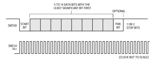
Figure 7-75. SMC UART Frame Format
