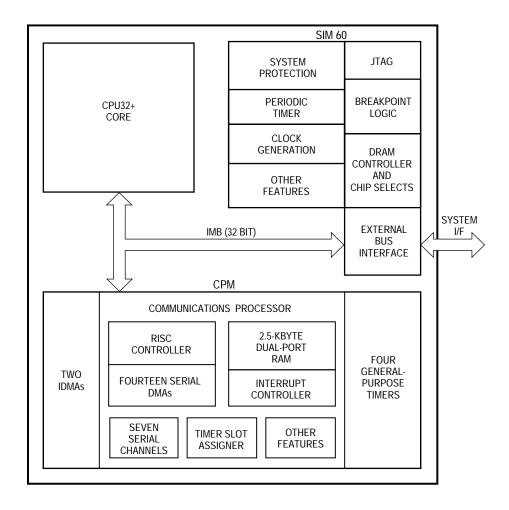
Figure D-1. QUICC Block Diagram
