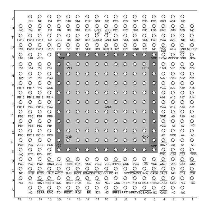
68360 OMPAC TOP VIEW 19 X 19 ARRAY 1.27mm PITCH
