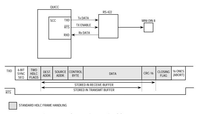
Figure 7-62. Connecting the QUICC to LocalTalk
