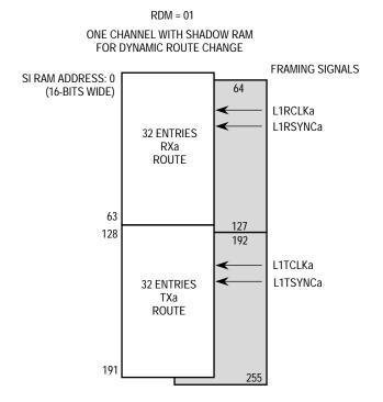
Figure 7-24. SI RAM: One TDM with Dynamic Frames
