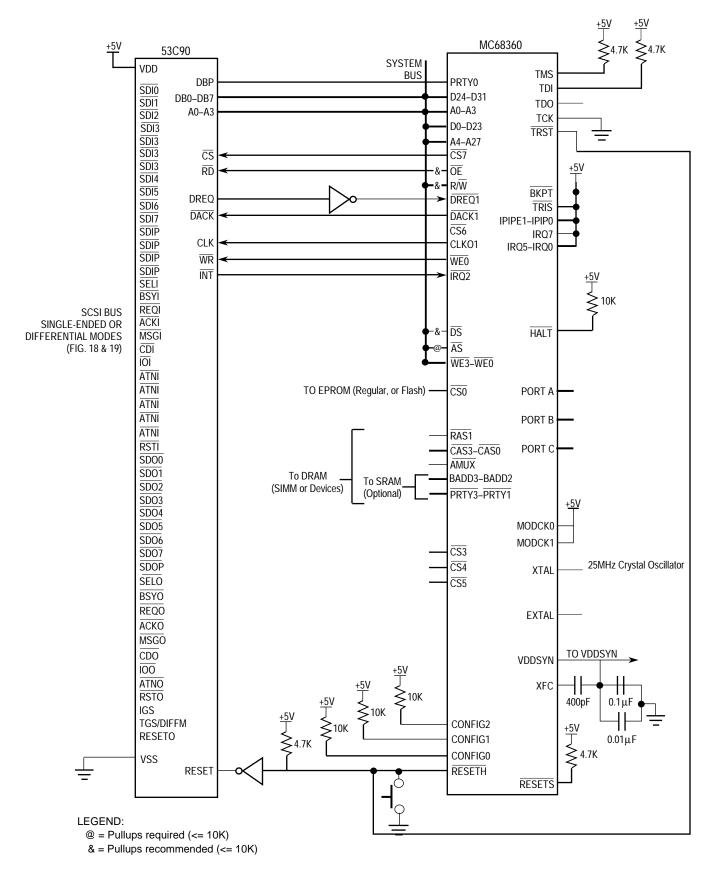
Figure 9-21. QUICC to SCSI Bus Interface
