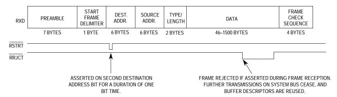
Figure 7-68. QUICC Ethernet Serial CAM Interface
