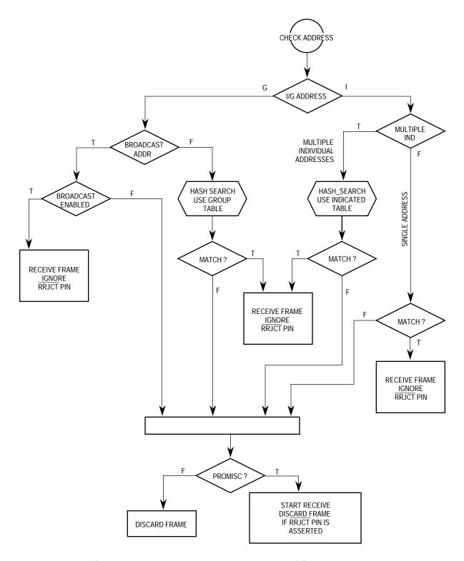
Figure 7-70. Ethernet Address Recognition Flowchart
