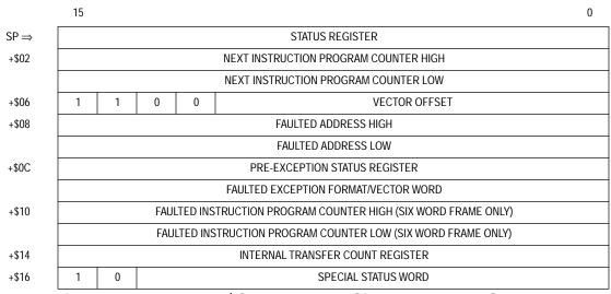
Figure 5-17. Format \$C—Four- and Six-Word BERR Stack
