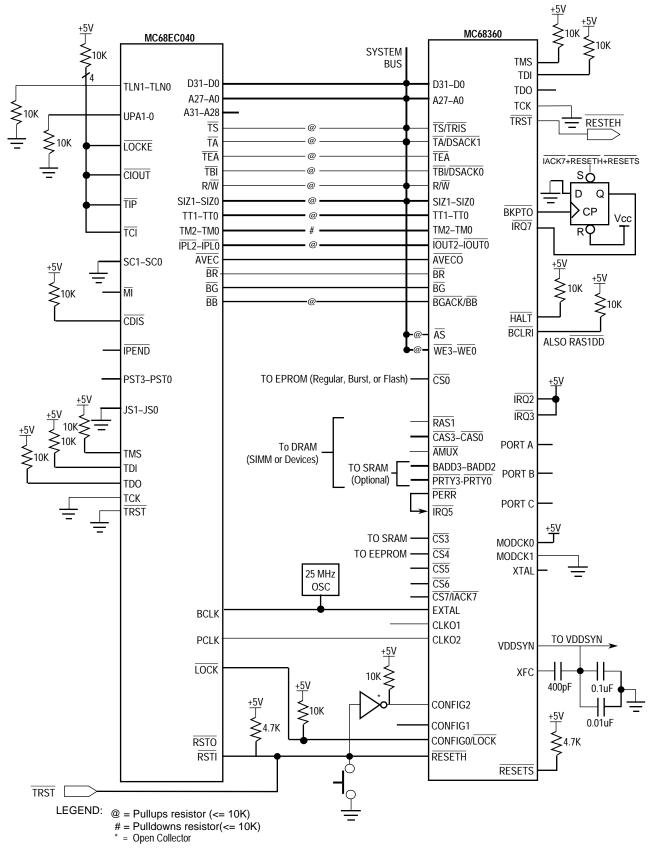
Figure 9-8. MC68EC040 to QUICC Interface
