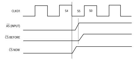
Figure 6-14. CSNTQ = 1 During an External QUICC/MC68EC030 Cycle
