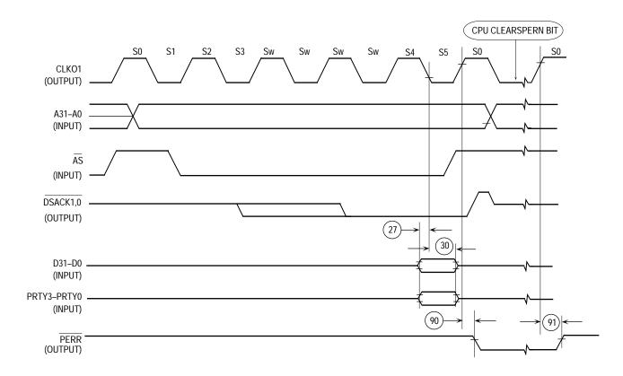
Figure 10-38. External MC68030/MC68360 Parity Bits Timing Diagram
