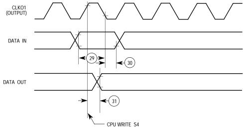
Figure 10-55. Parallel I/O Data-in/Data-Out Timing Diagram
