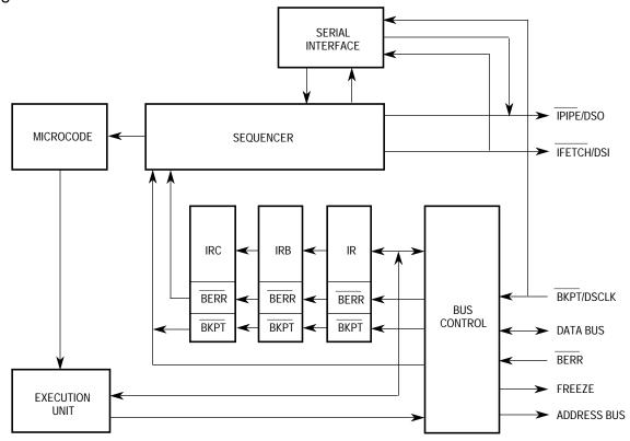
Figure 5-20. BDM Block Diagram
