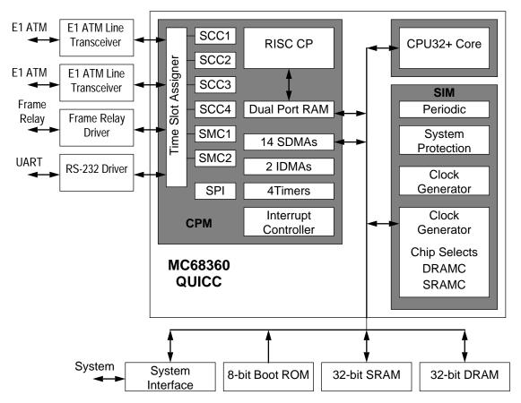
Figure C-2. ATM/Frame Relay Interwork System
