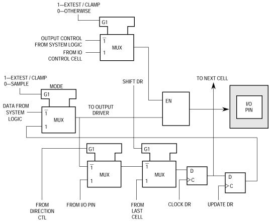
Figure 8-6. Bidirectional Data Cell (IO.Cell)
