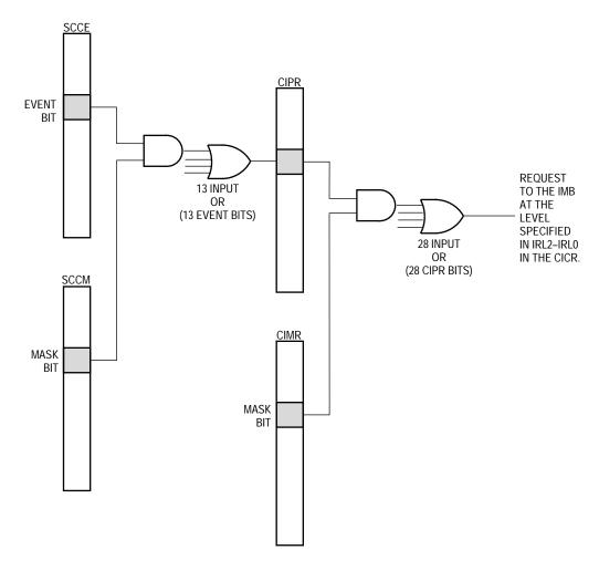
Figure 7-100. Interrupt Request Masking
