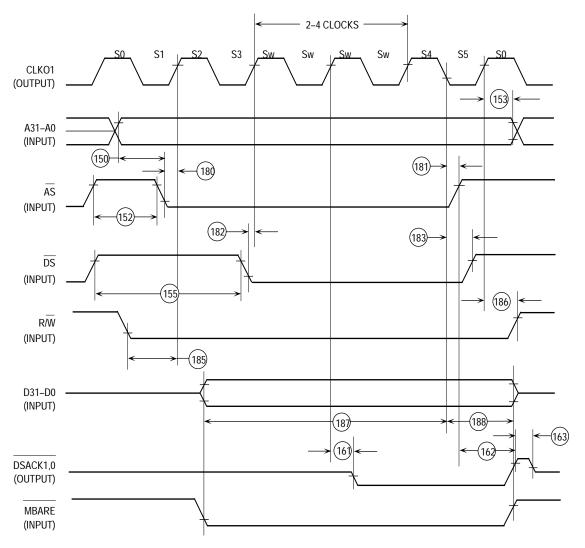
NOTE: Two wait states are inserted when writing to the SIM. Three wait states are inserted when writing to the dualport RAM and CPM. Four wait states are inserted when writing the SI RAM. Additional wait states may be inserted when the SHEN1–SHEN0 = 10 and one of the internal masters is accessing an internal peripheral.
