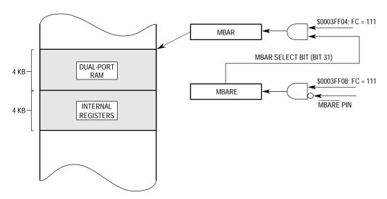
Figure 6-9. MBAR Access to a Multiple QUICC Slave System
