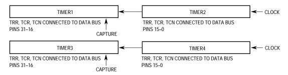
Figure 7-7. Timer Cascaded Mode Block Diagram
