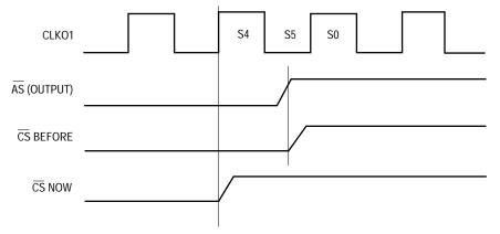
Figure 6-13. CSNTQ = 1 During an Internal Cycle
