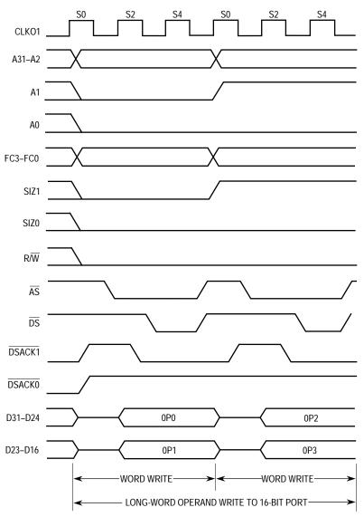
Figure 4-5. Long-Word Operand Write Timing (16-Bit Data Port)
