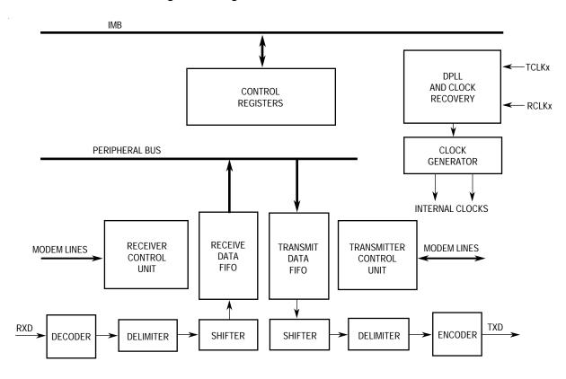
Figure 7-37. SCC Block Diagram
