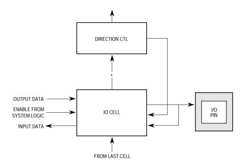
NOTE: More than one IO.Cell could be serially connected and controlled by a single IO.Ctl.
