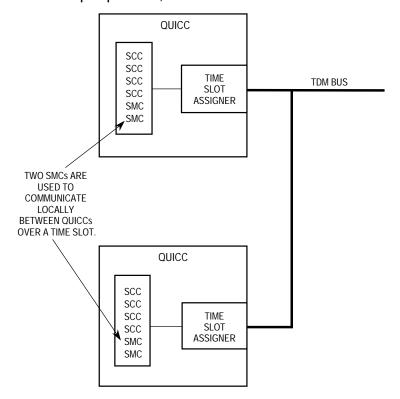
NOTE: The eight SCCs and two SMCs support 10 time slots on the TDM bus.
