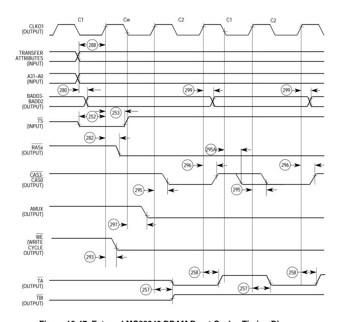
Figure 10-47. External MC68040 DRAM Burst Cycles Timing Diagram
