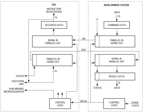
Figure 5-22. Debug Serial I/O Block Diagram
