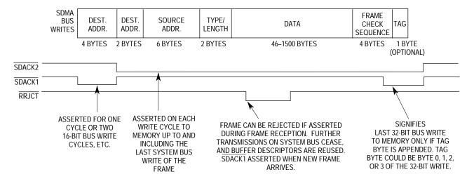
NOTE: The diagram shows SDMA system bus writes, not data on the RXD pin. Other bus activity may occur between successive 32-bit writes. In such a case, the SDACK2-1 pins would not be asserted for other bus activity.
