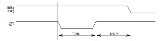
Figure 7-91. Centronics Receiver Timing Mode 2
