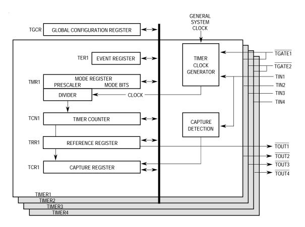
Figure 7-6. Timer Block Diagram
