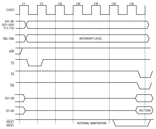
Figure 4-44. MC68EC040 Interrupt Acknowledge Cycle
