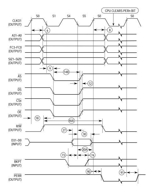
Figure 10-4. Fast Termination Read Cycle (Parity Check PAREN = 1, PBEE = 0)
