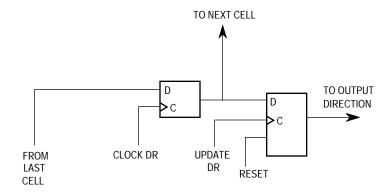
Figure 8-5. Control Cell (IO.Ctl)
