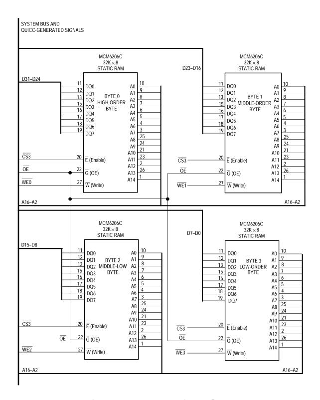
Figure 9-4. Glueless Interface to SRAM
