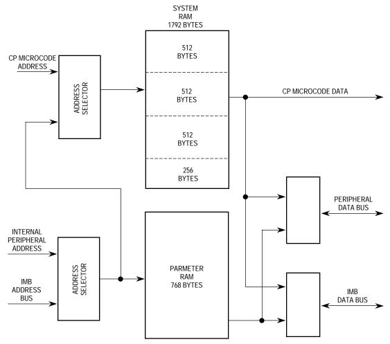
Figure 7-3. Dual-Port RAM Block Diagram
