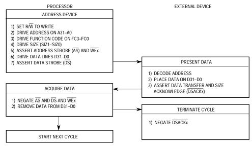
Figure 4-19. Write Cycle Flowchart
