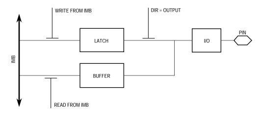
Figure 7-96. Port B General-Purpose I/O
