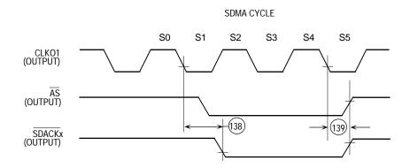
NOTE: SDACKx is asserted when the SDMA writes the received Ethernet frame into memory.
