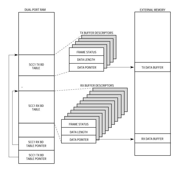
Figure 7-38. SCC Memory Structure
