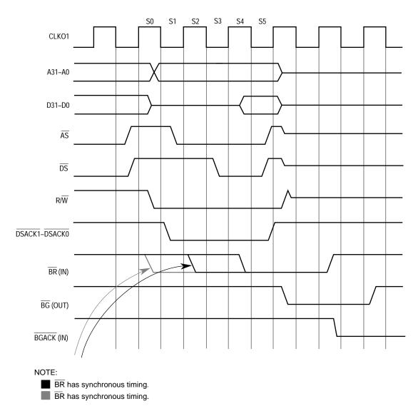
Figure 4-36. Bus Arbitration Timing Diagram—Active Bus Case
