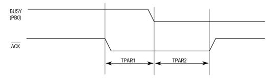
Figure 7-90. Centronics Receiver Timing Mode 1
