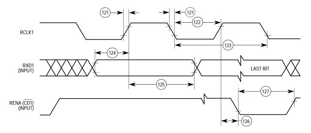
Figure 10-69. Ethernet Receive Timing
