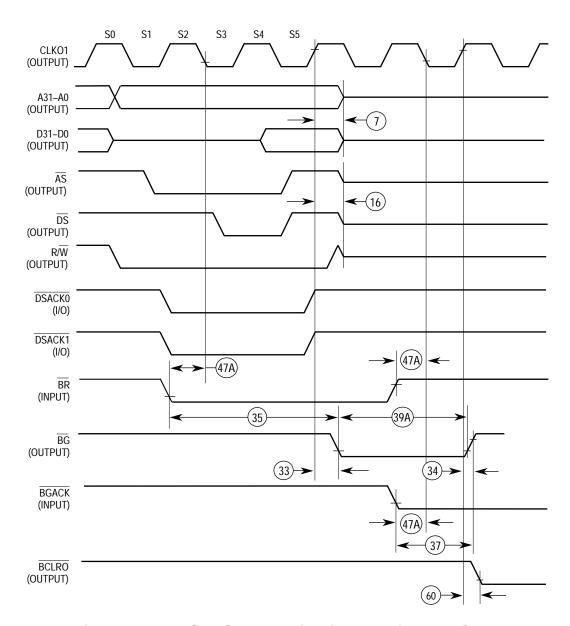
Figure 10-13. ASYNC Bus Arbitration – Active Bus Case
