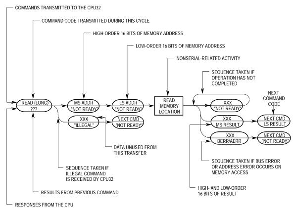
Figure 5-27. Command Sequence Diagram
