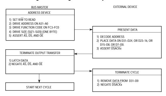
Figure 4-16. Byte Read Cycle Flowchart
