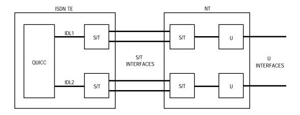
Figure 7-31. Dual IDL Bus Application Example
