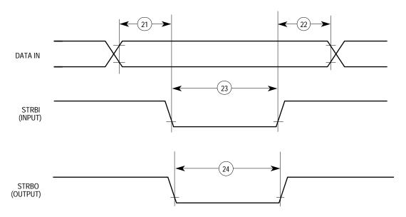
Figure 10-52. PIP Tx (Interlock Mode)
