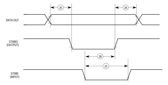
Figure 10-51. PIP Rx (Interlock Mode)
