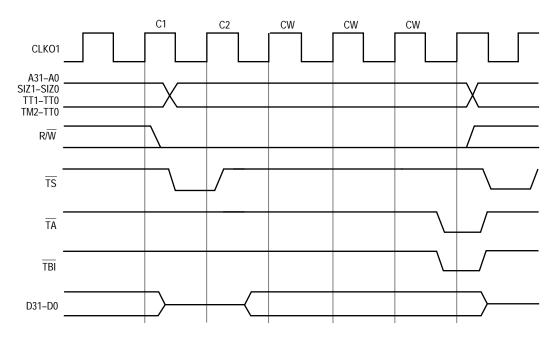
Figure 4-42. MC68EC040 Internal Registers Write Cycle
