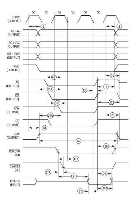
Figure 10-6. SRAM: Read Cycle (TRLX = 1)
