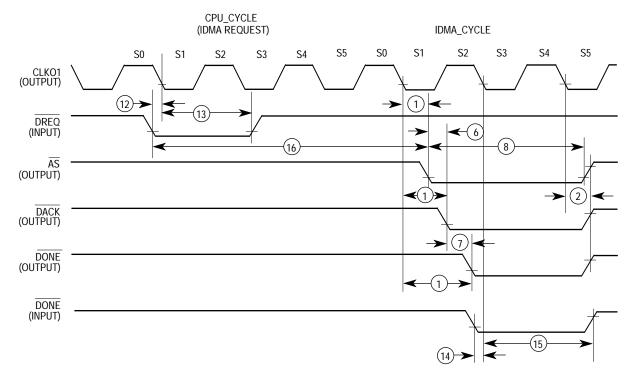
Figure 10-50. IDMA Signal Synchronous Timing diagram
