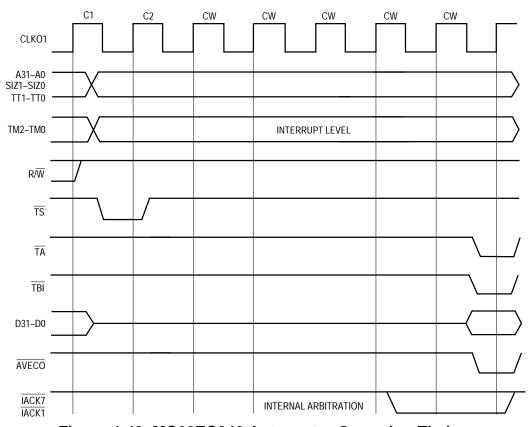
Figure 4-43. MC68EC040 Autovector Operation Timing
