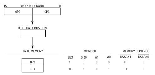
Figure 4-6. Example of Word Transfer to Byte Port
