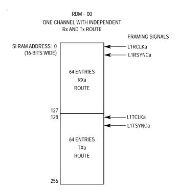
Figure 7-23. SI RAM: One TDM with Static Frames
