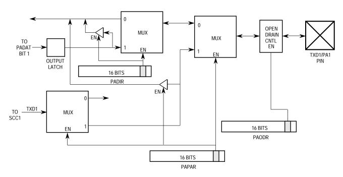
Figure 7-98. Parallel Block Diagram for PA1
