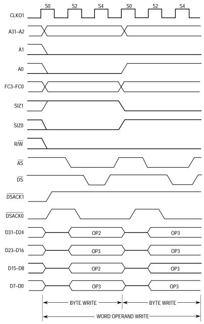
Figure 4-7. Word Operand Write Timing (8-Bit Data Port)
