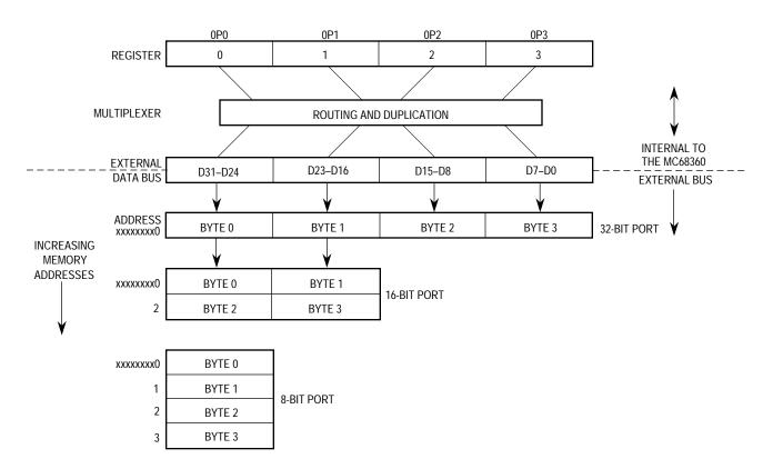
Figure 4-3. QUICC Interface to Various Port Sizes
