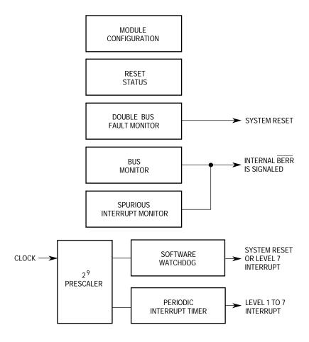
Figure 6-2. System Configuration and Protection Logic
