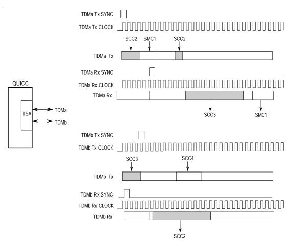
NOTE: SCCs may receive on one TDM and transmit on another (e.g., SCC2 and SCC3).
