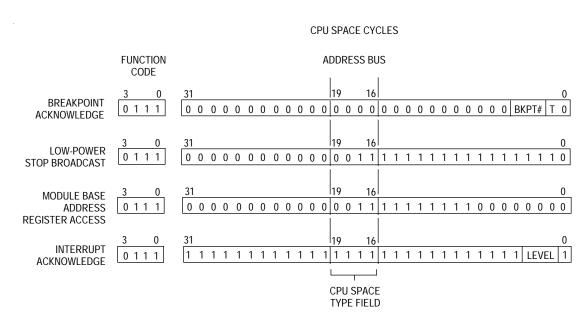
Figure 4-22. CPU Space Address Encoding
