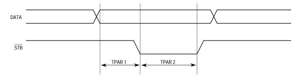
Figure 7-88. Centronics Transmitter Timing
