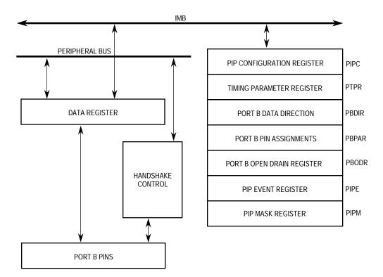
Figure 7-84. PIP Block Diagram
