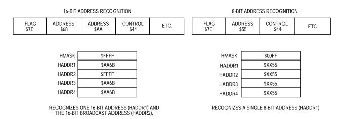
Figure 7-51. HDLC Address Recognition Example
