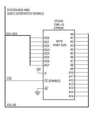
Figure 9-2. Glueless Interface to Standard EPROM
