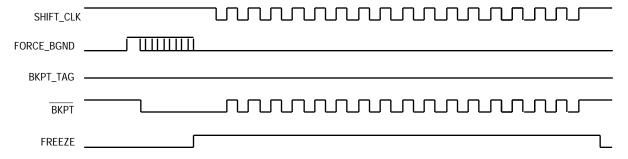
Figure 5-25. BKPT Timing for Forcing BDM
