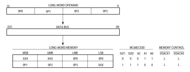
Figure 4-12. Misaligned Long-Word Transfer to Long-Word Port Example
