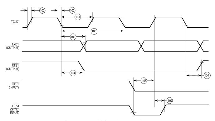
Figure 10-66. SCC NMSI Transmit
