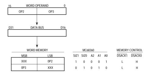
Figure 4-10. Misaligned Word Transfer to Word Port Example
