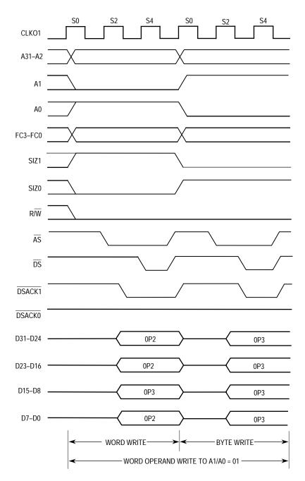
Figure 4-11. Misaligned Word Transfer to Word Port Timing
