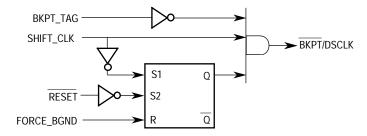
Figure 5-26. BKPT/DSCLK Logic Diagram
