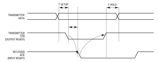
Figure 7-85. Interlock Handshake Mode
