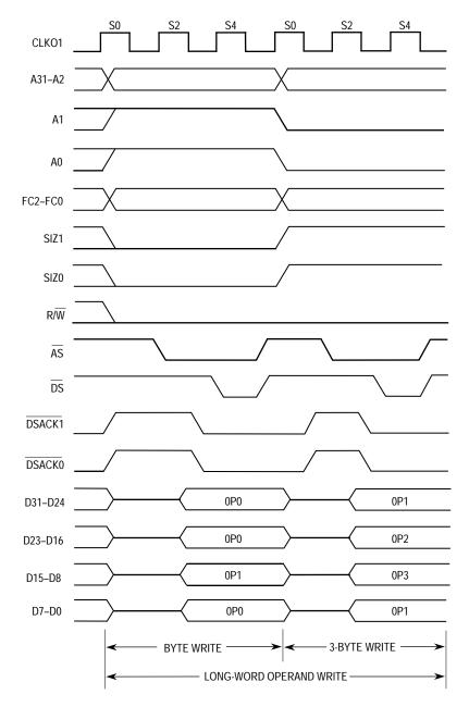
Figure 4-13. Misaligned Long-Word Transfer to Long-Word Port Timing
