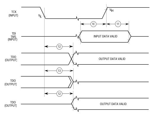
Figure 10-82. Test Access Port Timing Diagram
