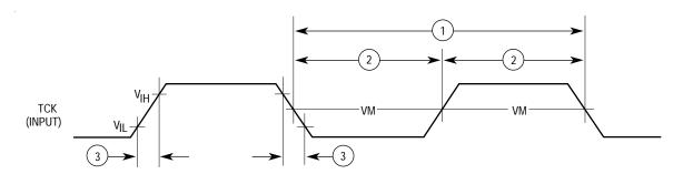
Figure 10-79. Test Clock Input Timing Diagram
