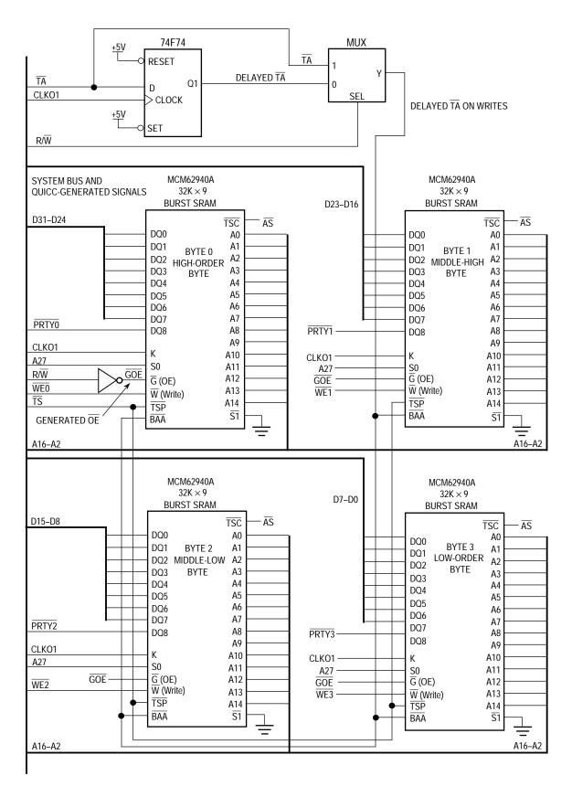
Figure 9-13. 128-Kbyte Burst SRAM Bank—32 Bits Wide
