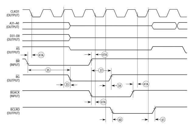
Figure 10-12. ASYNC Bus Arbitration – IDLE Bus Case
