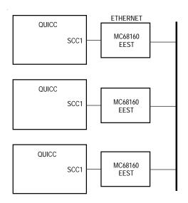
Figure 1-4. Ethernet LAN Capability
