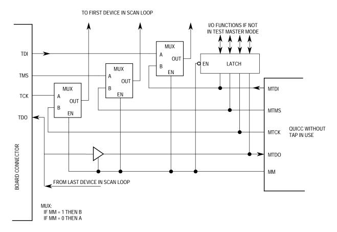
Figure 9-25. Signal Routing for Test Bus Master
