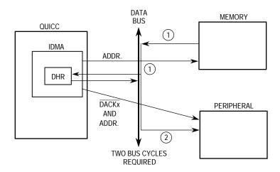
Figure 7-13. Dual Address Transfer Example
