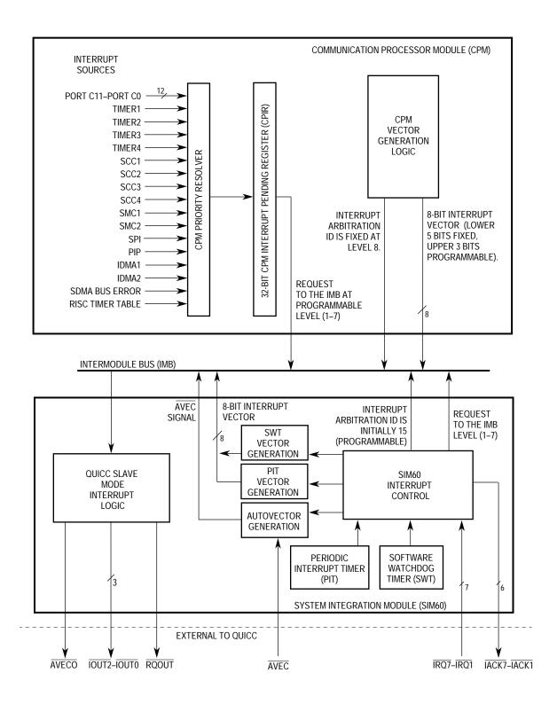
Figure 7-99. QUICC Interrupt Structure
