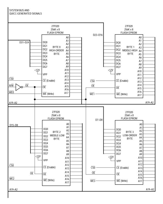
Figure 9-29. F1-Mbyte Flash EPROM Bank—32 Bits Wide
