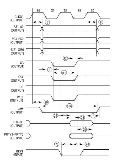
Figure 10-9. Fast Termination Write Cycle
