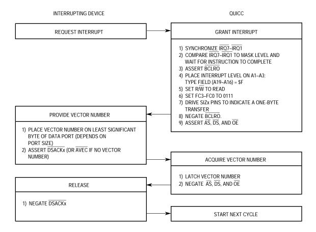
Figure 4-26. Interrupt Acknowledge Cycle Flowchart
