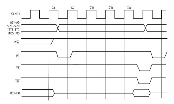
Figure 4-41. MC68EC040 Internal Registers Read Cycle
