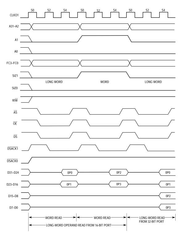
Figure 4-18. Long-Word Read—16-Bit and 32-Bit Port Timing
