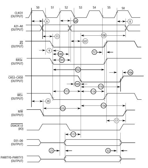
Figure 10-21. DRAM: Normal Write Cycle
