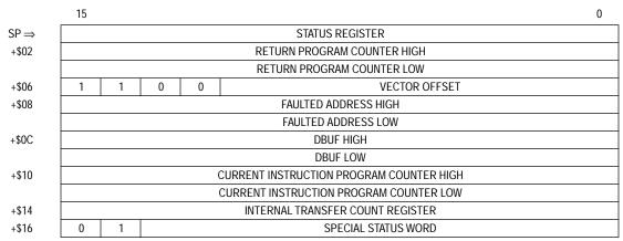
Figure 5-16. Format \$C—BERR Stack on MOVEM Operand
