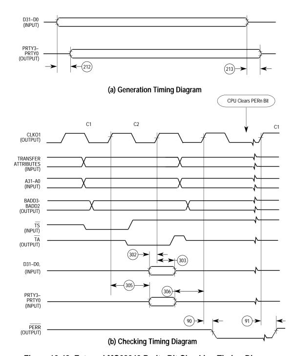
Figure 10-48. External MC68040 Parity Bit Checking Timing Diagram
