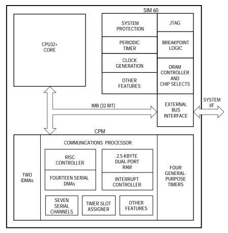
Figure 1-1. QUICC Block Diagram
