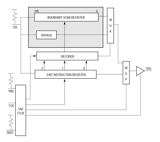
Figure 8-1. Test Logic Block Diagram
