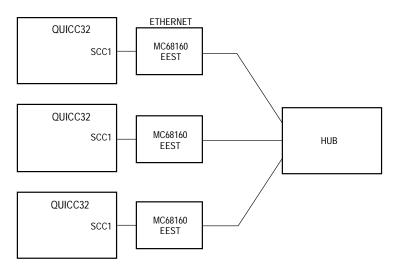
Figure D-2. Ethernet LAN Capability
