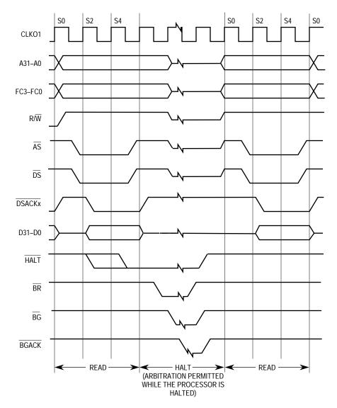
Figure 4-33. HALT Timing
