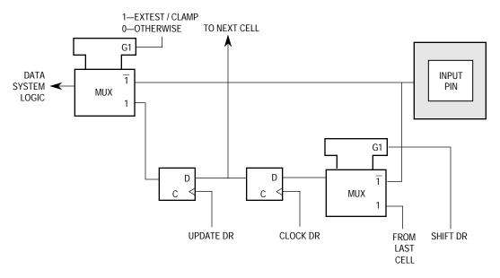
Figure 8-4. Input Pin Cell (I.Pin)
