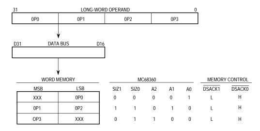
Figure 4-8. Misaligned Long-Word Transfer to Word Port Example
