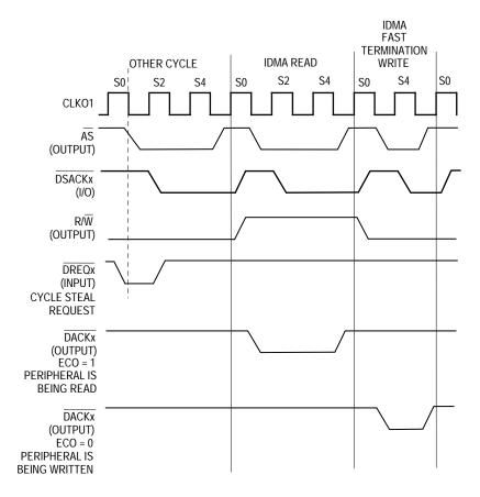
NOTE: This example shows a fast termination on the write cycle. The fast termination may occur on the read, write, or both.
