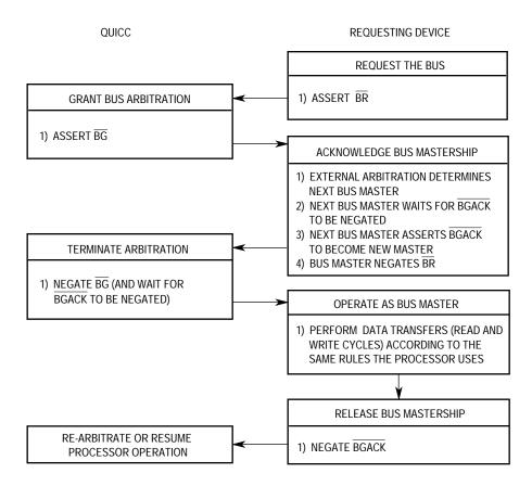
Figure 4-34. Bus Arbitration Flowchart for Single Request
