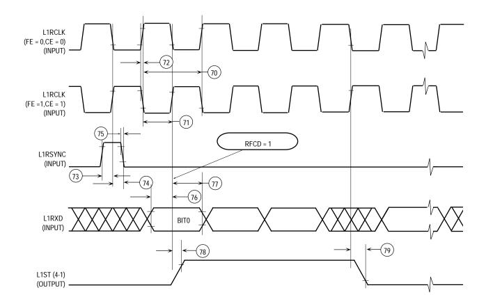
Figure 10-60. SI Receive Timing with Normal Clocking (DSC = 0)
