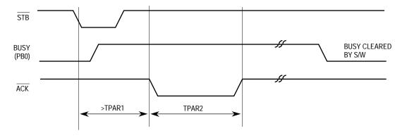
Figure 7-92. Centronics Receiver Timing Mode 3
