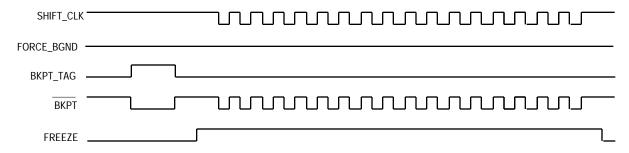
Figure 5-24. BKPT Timing for Single Bus Cycle
