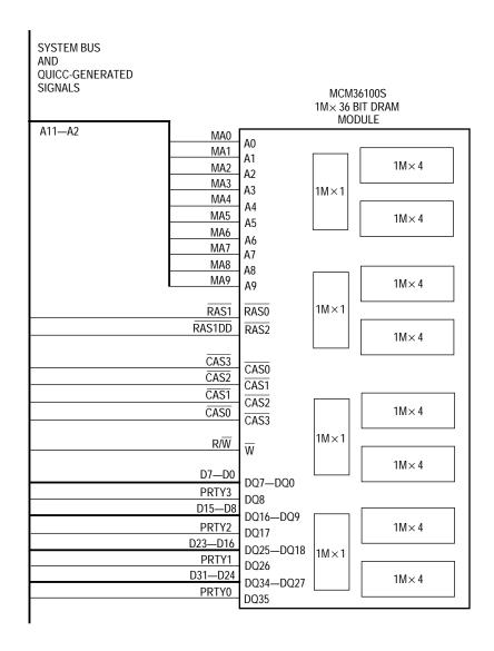
Figure 9-6. Glueless Interface to MCM36100S SRAM
