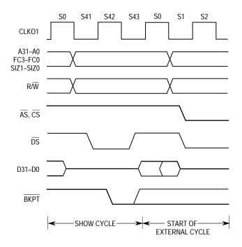
Figure 4-45. Show Cycle Timing Diagram
