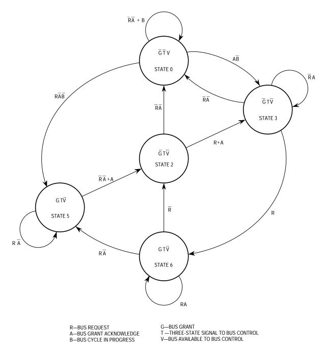
Figure 4-37. Bus Arbitration State Diagram
