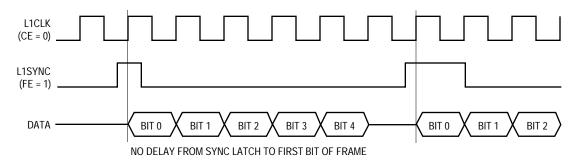
Figure 7-30. No Delay from Sync to Data (RFSD = 00)
