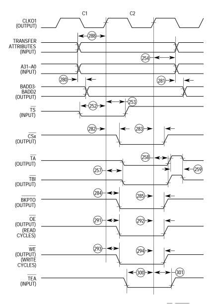
NOTE: MC68040 Transfer Attribute Signals = SIZx, TTx, TMx, R/W, LOCK
