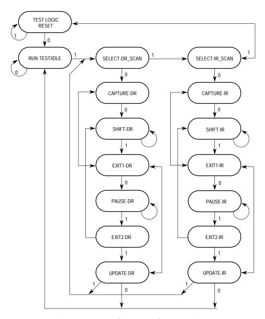
Figure 8-2. TAP Controller State Machine
