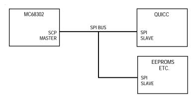
NOTE: The MC68302 SCP can communicate with the QUICC SPI.
