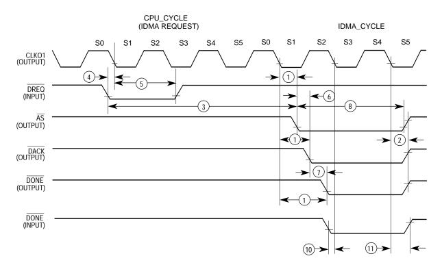
Figure 10-49. IDMA Signal Asynchronous Timing diagram
