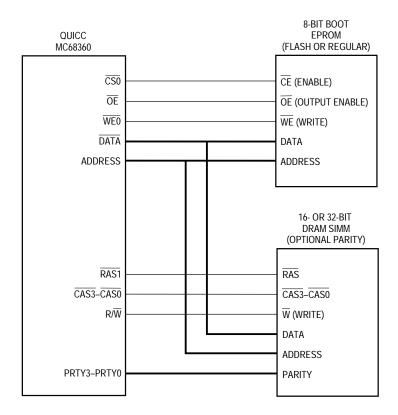
Figure 1-2. Minimum QUICC System Configuration
