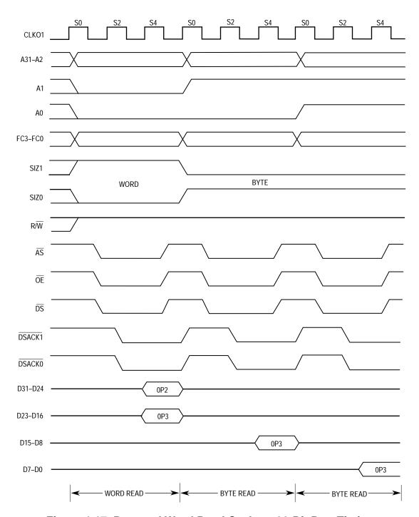
Figure 4-17. Byte and Word Read Cycles—32-Bit Port Timing
