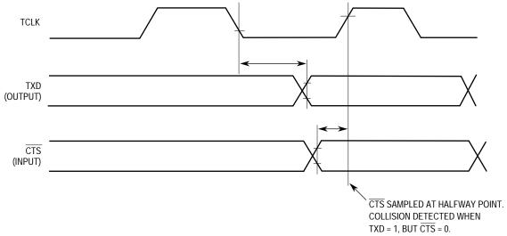
Figure 7-56. HDLC Bus Collision Detection
