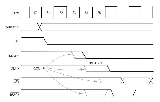
Figure 6-17. TRLXQ = 1 During an External QUICC/MC68030 Cycle
