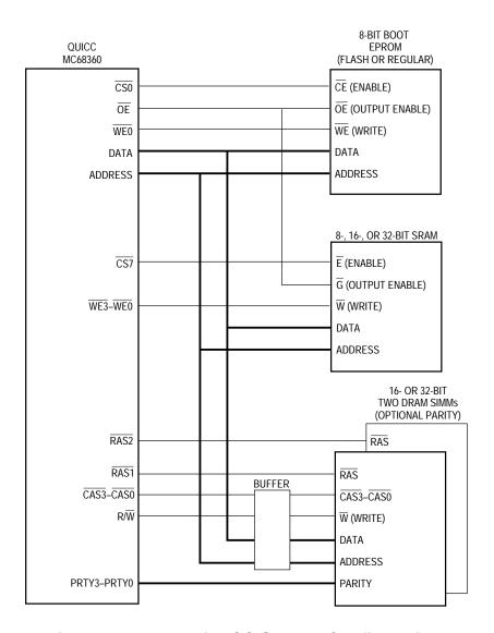
Figure 1-3. Larger QUICC System Configuration
