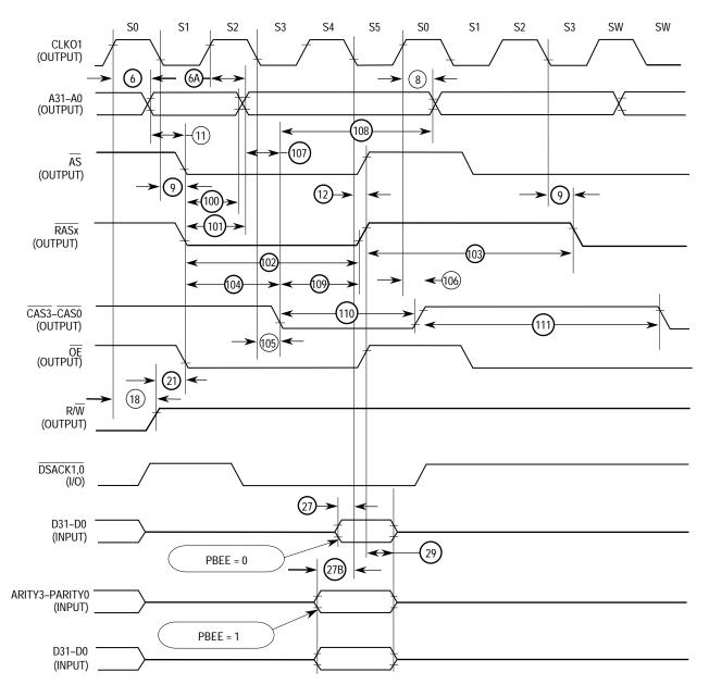
Figure 10-20. DRAM: Normal Read Cycle (Internal Mux, TRLX = 0)
