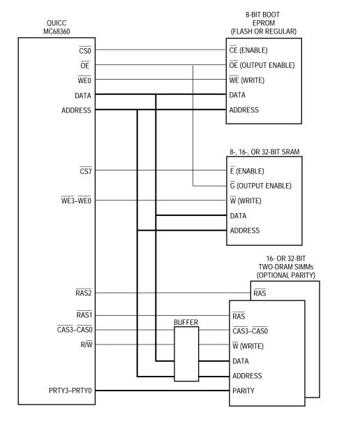
Figure 6-12. Larger QUICC System Configuration
