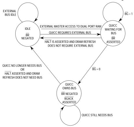
NOTE: BGACK is only asserted by QUICC during the state "QUICC Owns Bus", otherwise BGACK is three-stated by the QUICC.
