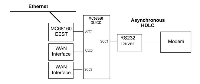
Figure C-3. Asynchronous HDLC Block Diagram
