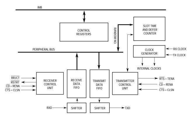
Figure 7-66. Ethernet Block Diagram
