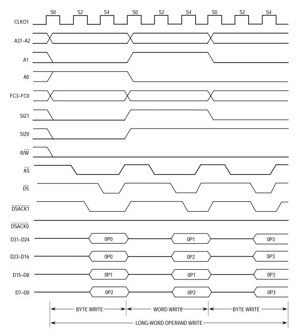
Figure 4-9. Misaligned Long-Word Transfer to Word Port Timing
