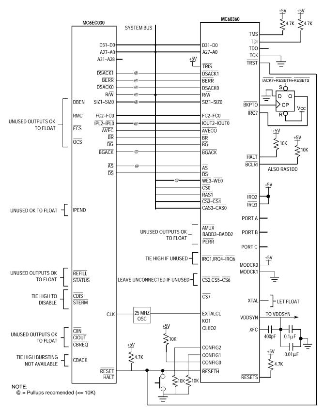
Figure 9-27. MC68EC030 to QUICC Interface
