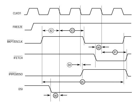
Figure 10-19. Background Debug Mode Serial Port Timing
