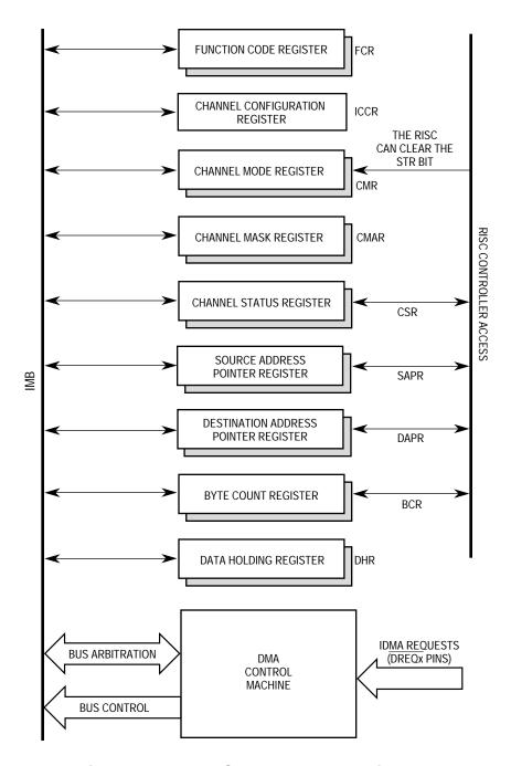
Figure 7-8. IDMA Controller Block Diagram
