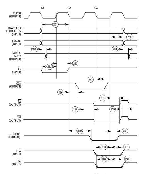
NOTE: MC68040 Transfer Attribute Signals = SIZx, TTx, TMx, R/W, LOCK
