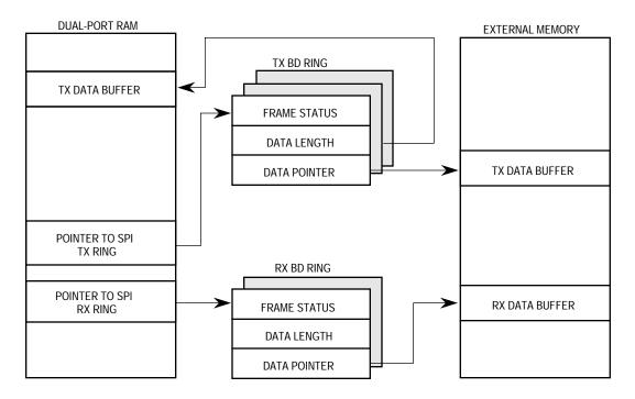
Figure 7-83. SPI Memory Structure
