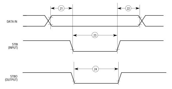
Figure 10-53. PIP Tx (Pulse Mode)
