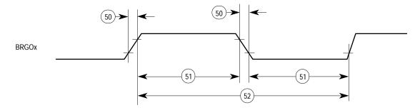
Figure 10-58. Baud Rate Generator Output Signals
