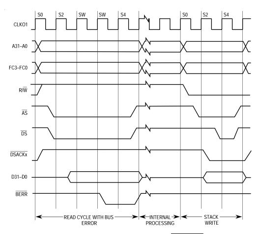
Figure 4-29. Bus Error without DSACKx
