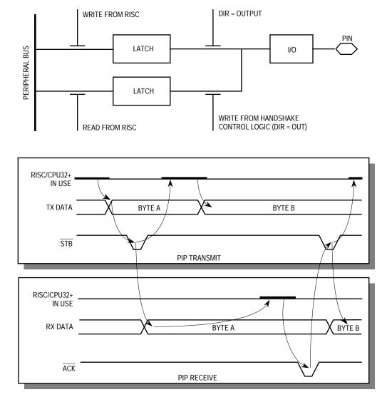
Figure 7-86. Pulsed Handshake Full Cycle
