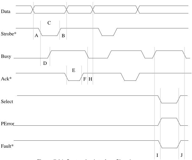
Figure 7-94. Centronics Interface Signals
