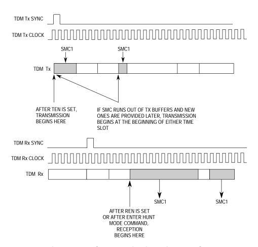
Figure 7-79. Synchronization with the TSA
