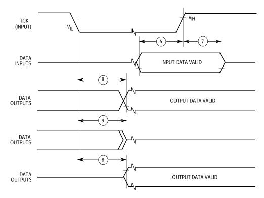
Figure 10-81. Boundary Scan (JTAG) Timing Diagram
