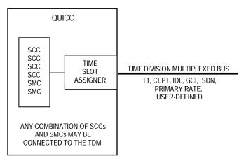
NOTE: Independent receive and transmit clocking, routing, and syncs are supported.
