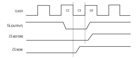
Figure 6-15. CSNT40 = 1 During an External MC68EC040 Cycle
