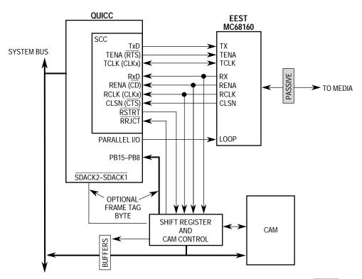
NOTE: The receive data is sent directly from the EE<u>ST serial</u> interface to the CAM using RXD and RCLK. RSTRT is asserted at the beginning of the destination address. RRJCT should be asserted during the frame to cause the frame to be rejected. The system bus is used for CAM initialization and maintenance.
