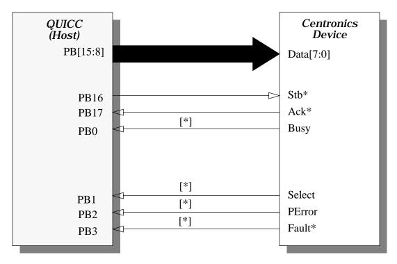
[\*] - optional Figure 7-95. Centronics Transmitter Configuration
