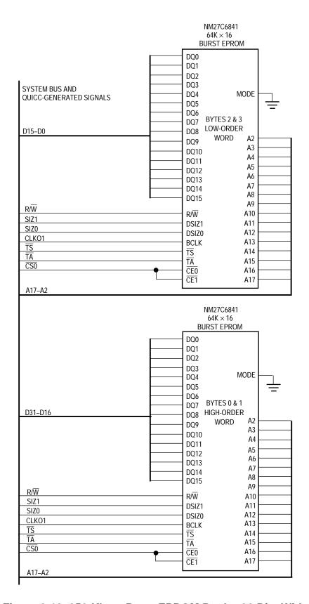
Figure 9-10. 256-Kbyte Burst EPROM Bank—32 Bits Wide
