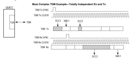
Figure 7-20. Various Configurations of a Single TDM Channel
