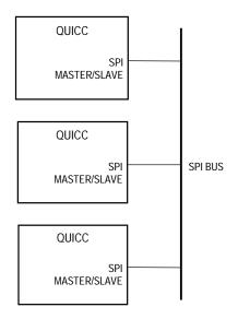
NOTE: SPI bus configuration—each QUICC can be the master in turn.
