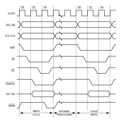
Figure 4-30. Late Bus Error with DSACKx
