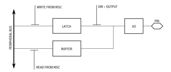
Figure 7-93. PIP Transparent Handshake Mode
