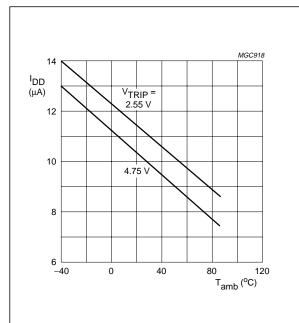
Fig.4 Supply current as a function of temperature;  $V_{DD} = 5 \text{ V}$ ; COMIN =  $V_{DD}$ .
