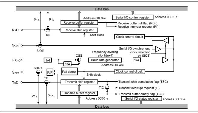
Fig. 8 Clock synchronous serial I/O block diagram
