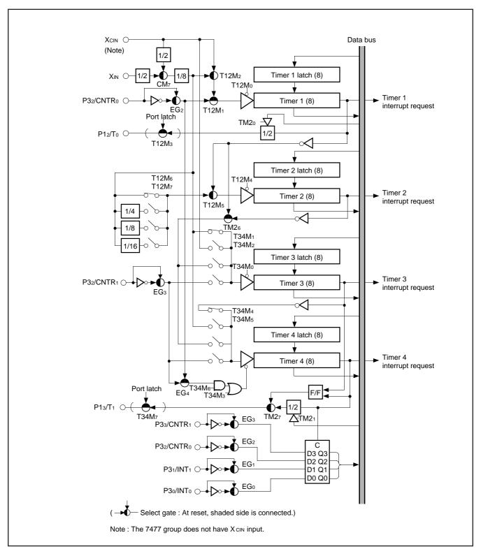
Fig. 6 Block diagram of timer 1 through 4
