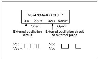
Fig. 26 External clock input circuit (7478 group)
