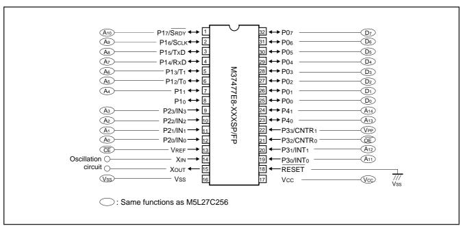
Fig. 32 Pin connection in EPROM mode
