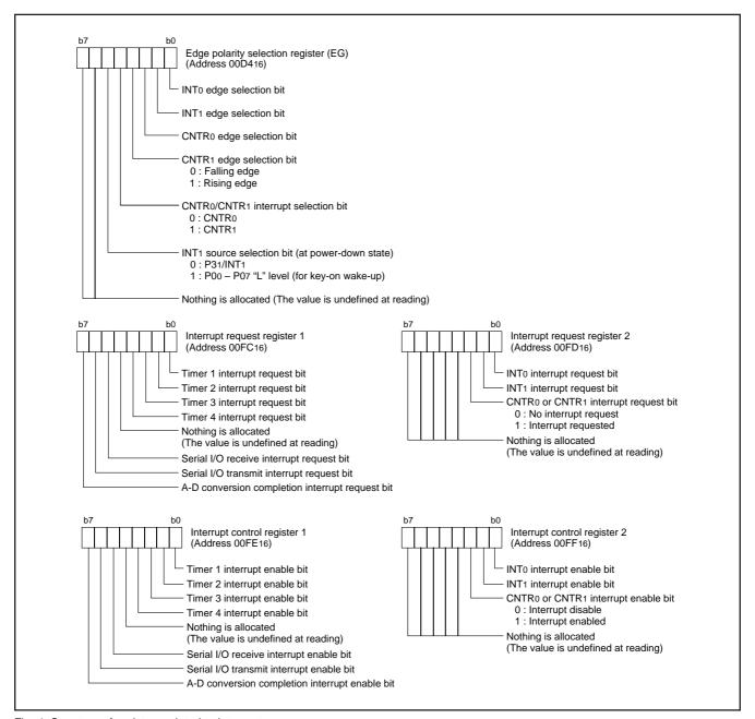
Fig. 4 Structure of registers related to interrupt
