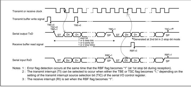
Fig. 11 Operation of UART serial I/O function
