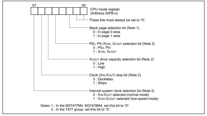
Fig. 28 Structure of CPU mode register
