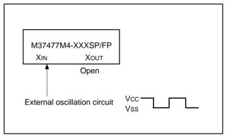
Fig. 25 External clock input circuit (7477 group)
