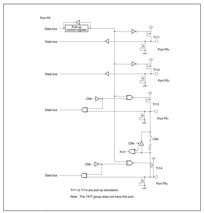
Fig. 22 Block diagram of port P5
