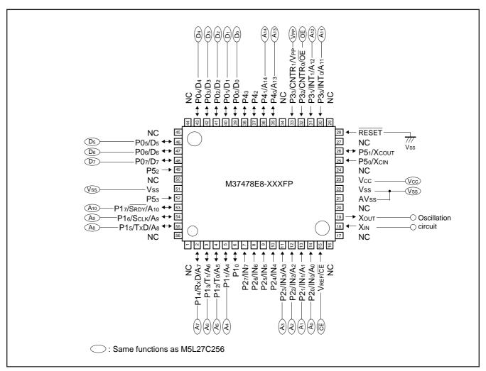
Fig. 31 Pin connection in EPROM mode
