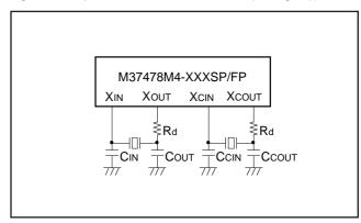
Fig. 24 Example of ceramic resonator circuit (7478 group)
