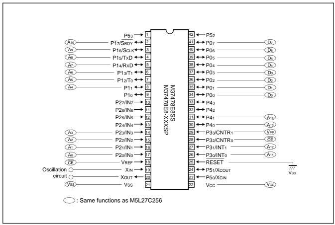
Fig. 30 Pin connection in EPROM mode
