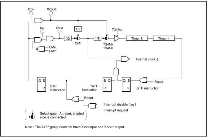
Fig. 27 Block diagram of clock generating circuit
