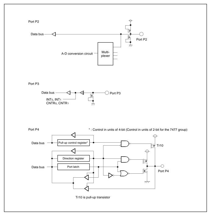
Fig. 21 Block diagram of ports P2 - P4
