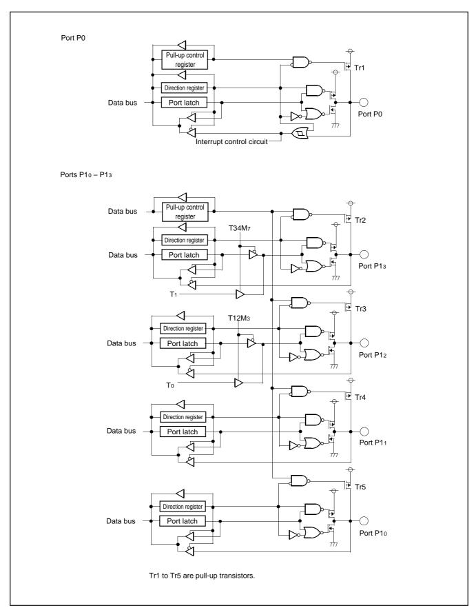
Fig. 19 Block diagram of ports P0, P10-P13
