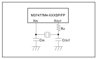
Fig. 23 Example of ceramic resonator circuit (7477 group)
