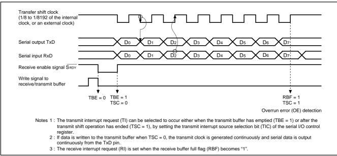
Fig. 9 Operation of clock synchronous serial I/O function
