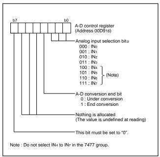
Fig. 14 Structure of A-D control register
