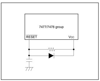
Fig. 16 Example of reset circuit
