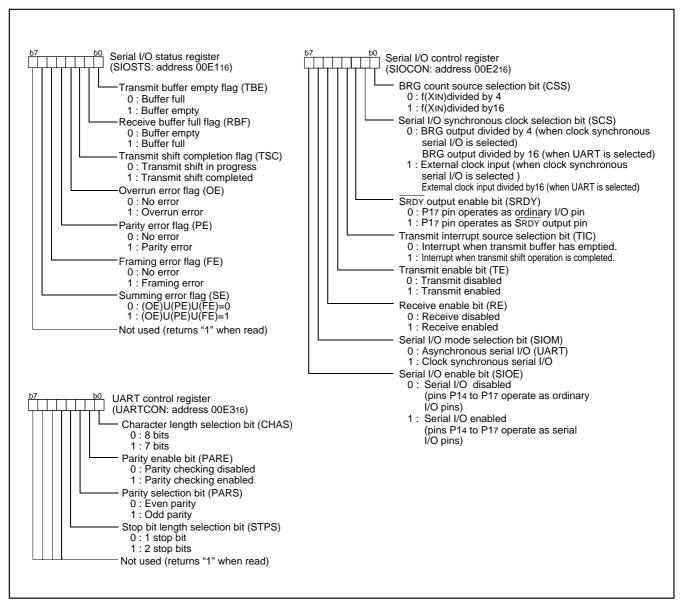
Fig. 12 Structure of serial I/O control registers
