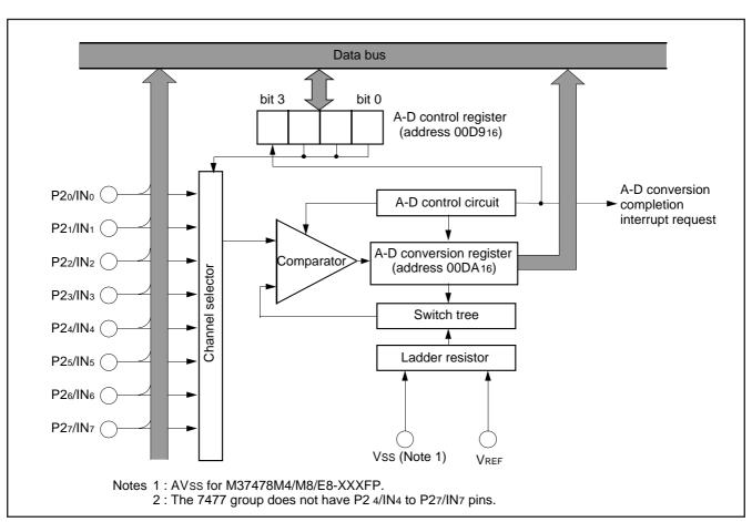
Fig. 13 A-D converter circuit
