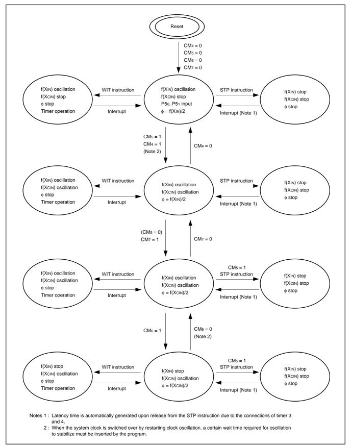
Fig. 29 Transition of states for the system clock.
