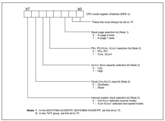
Fig. 1 Structure of CPU mode register
