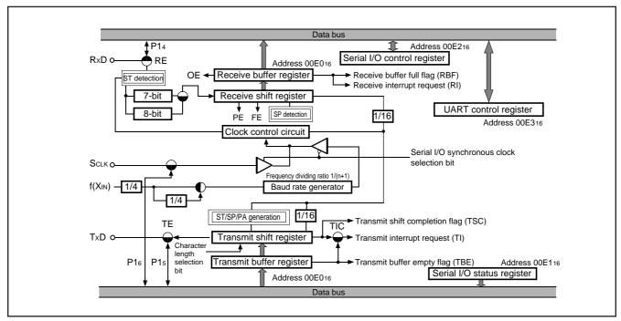
Fig. 10 UART serial I/O block diagram
