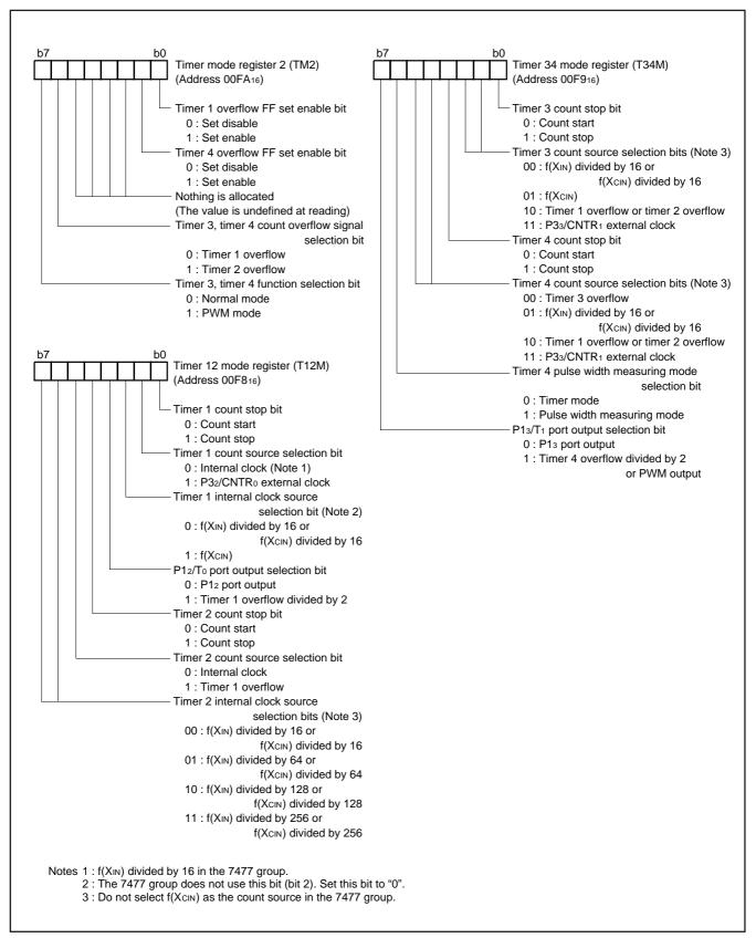
Fig. 7 Structure of timer mode registers
