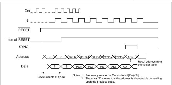
Fig. 18 Timing diagram at reset
