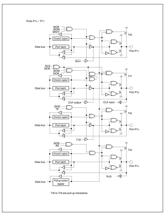
Fig. 20 Block diagram of ports P14 - P17
