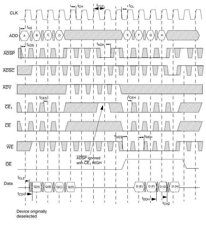
$\overline{CE}$  is the combination of  $CE_2$  and  $\overline{CE}_3$ . All chip selects need to be active in order to select the device. RAx stands for Read Address X, WAx stands for Write Address X, Dx stands for Data-in X, Qx stands for Data-out X.
