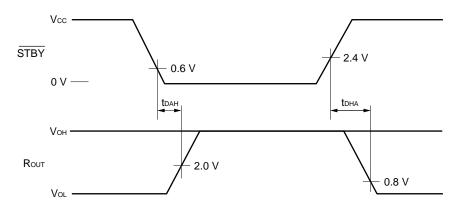
Receiver outputs are indefinite during transition time (tDHA).
