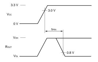
Receiver outputs are indefinite during reset release time (tPRA).
