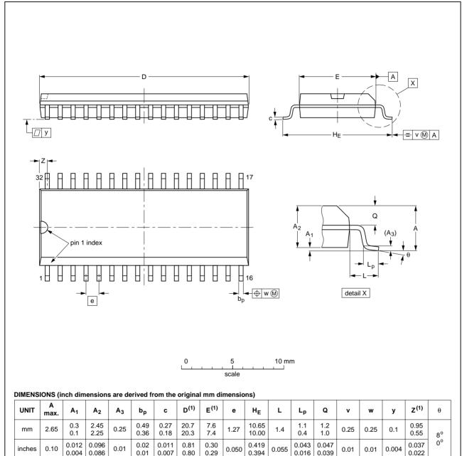
1. Plastic or metal protrusions of 0.15 mm maximum per side are not included.
