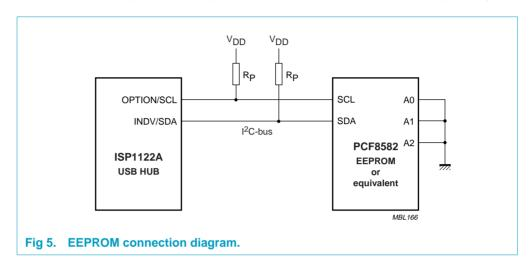
The slave address which ISP1122A uses to access the EEPROM is 1010000B. Page mode addressing is not supported, so pins A0, A1 and A2 of the EEPROM must be connected to GND (logic 0).
