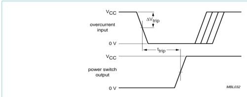
Overcurrent input: OCn; power switch output: PSWn.
