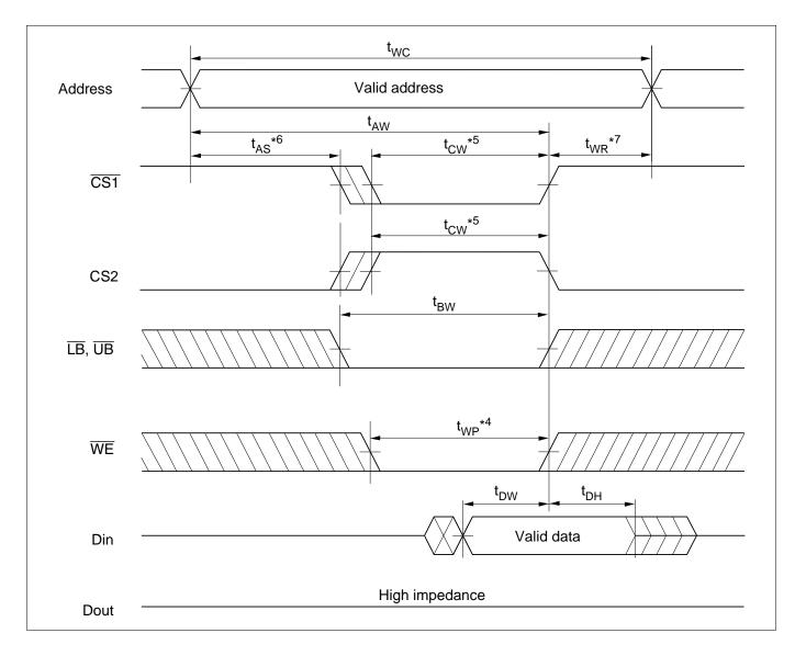
Write Cycle (3) ( $\overline{\text{LB}}$ ,  $\overline{\text{UB}}$  Clock,  $\overline{\text{OE}} = V_{\text{IH}}$ )
