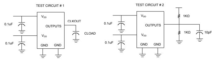
For parameter  $t_8$  (output skew rate) on -1H devices
