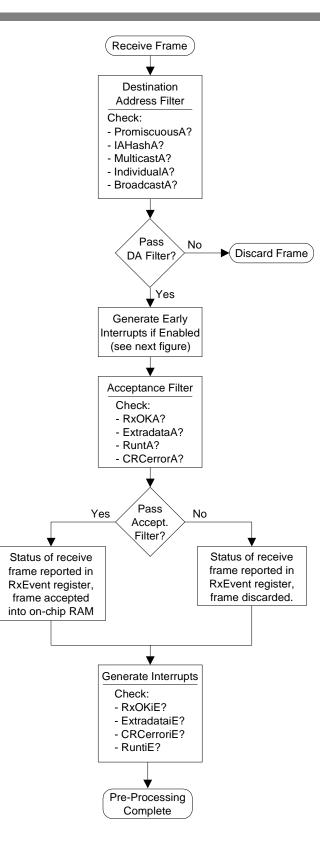
Figure 20. Receive Frame Pre-Processing
