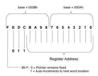
Figure 22. Ethernet Port Pointer
