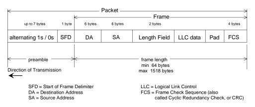
Figure 13. Ethernet Frame Format
