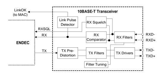
Figure 17. 10BASE-T Transceiver
