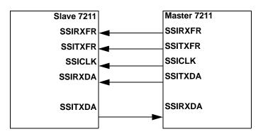
Figure 9. SSI2 Port Directions in Slave and Master Mode
