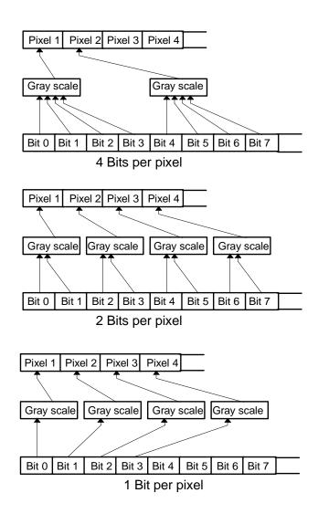
Figure 11. Video Buffer Mapping
