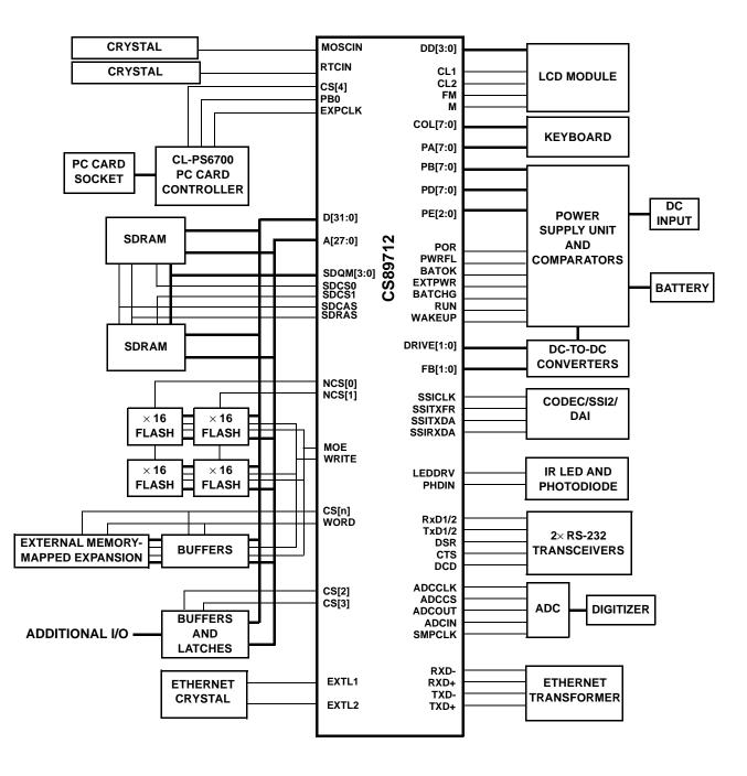
Figure 1. A CS89712–Based System
