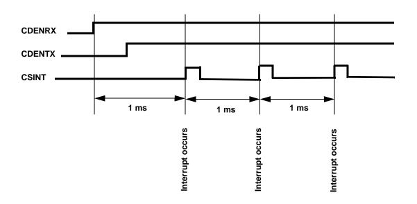
Figure 5. Codec Interrupt Timing
