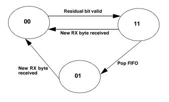
Figure 10. Residual Byte Reading
