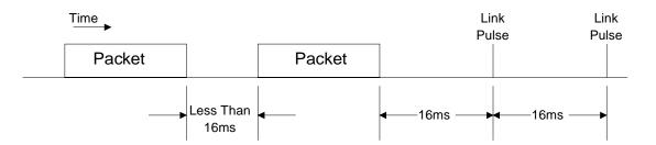
Figure 18. Link Pulse Transmission
