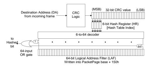
Figure 21. Hash Filter Operation
