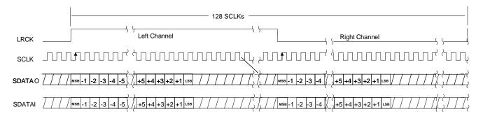
Figure 8. CS89712 - Digital Audio Interface Timing – MSB / Left Justified format
