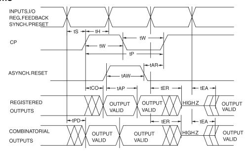
Note: 1. Timing measurement reference is 1.5V. Input AC driving levels are 0.0V and 3.0V, unless otherwise specified.
