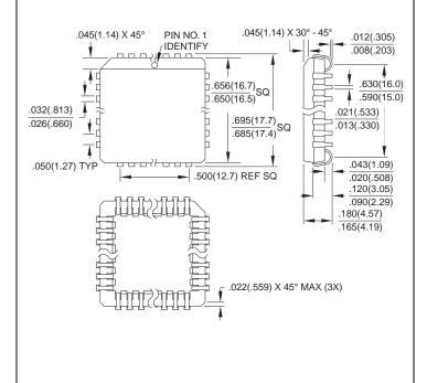
44KW, 44-Lead, Windowed, Ceramic J-Leaded Chip Carrier (JLCC)
