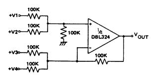
$$V_{OUT} = V1 + V2 - V3 - V4$$
