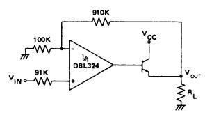
$$V_{OUT} = 0V \text{ for } V_{IN} = 0V$$
