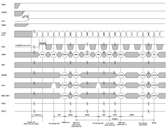
$\mbox{$^{\star}$}$  200 cycle(tXSRD) of CK are required (for DLL locking) before Read Command
