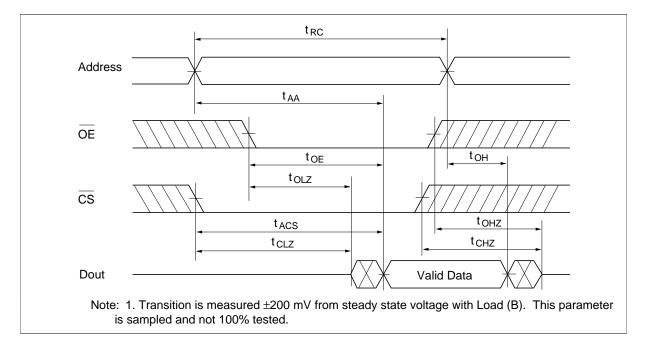
Read Timing Waveform (2)  $^{*1}(\overline{WE} = V_{II}, \overline{CS} = V_{IL}, \overline{OE} = V_{IL})$
