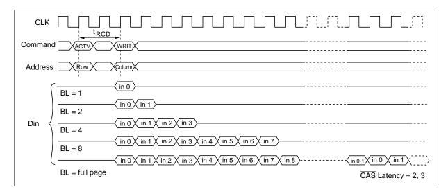
**2. Single write:** A single write operation is enabled by setting OPCODE (A9, A8) to (1, 0). In a single write operation, data is only written to the column address (AY0 to AY7; HM5264165F, AY0 to AY8; HM5264805F, AY0 to AY9; HM5264405F) and the bank select address (A12/A13) specified by the write command set cycle without regard to the burst length setting. (The latency of data input is 0 clock).
